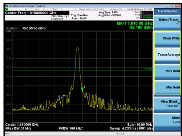
LTE-M Band 2 5MHz QPSK 100%RB CH-High
