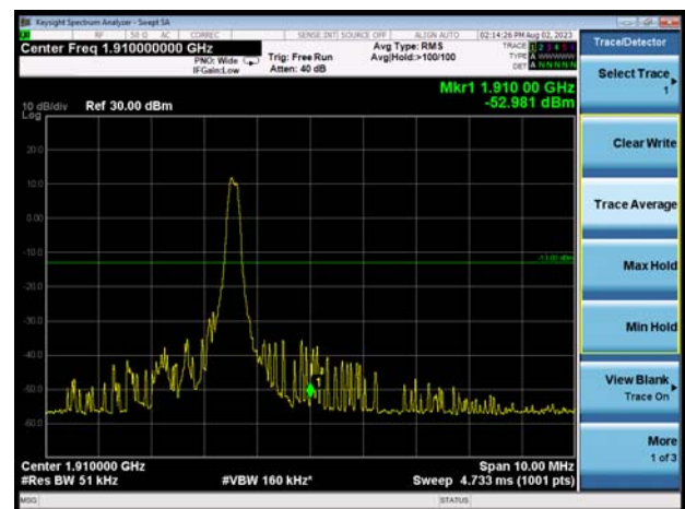
LTE-M Band 2 20MHz 16QAM 100%RB CH-High
