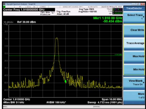
LTE-M Band 2 10MHz 16QAM 100%RB CH-High
