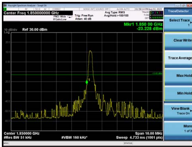
LTE-M Band 2 1.4MHz 16QAM 100%RB CH-Low
