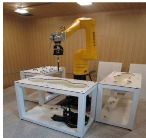
Figure E.7.1 DASY5 Test System
