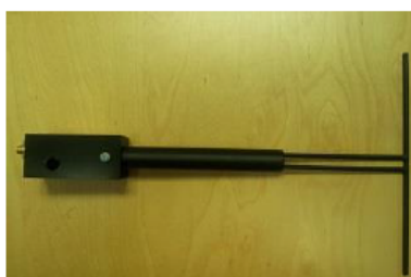
Figure 1 – MVG COMOSAR Validation Dipole
