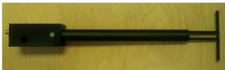
Figure 1 – MVG COMOSAR Validation Dipole
