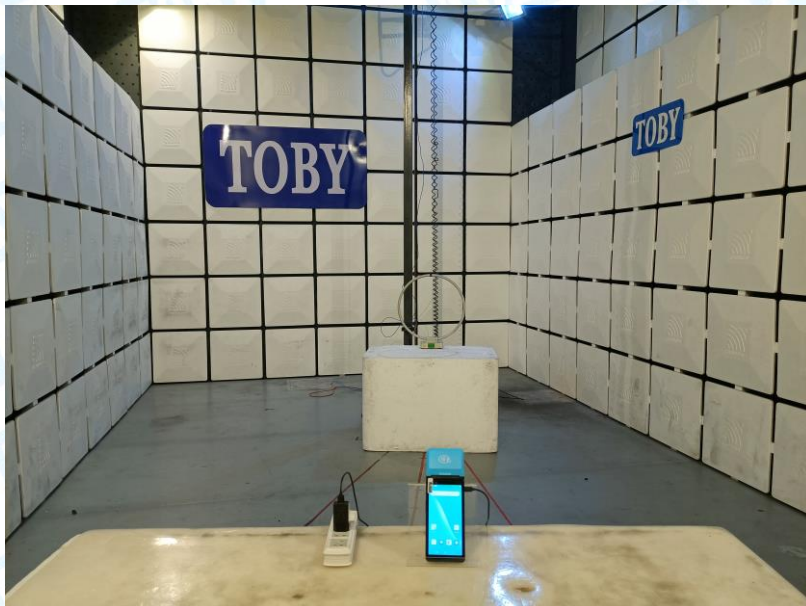
Photo of Setup for Conducted Emission
