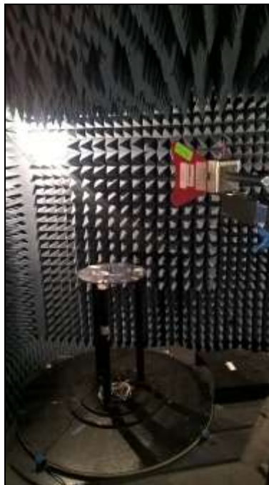
Photograph 1. Radiated Spurious Emissions, Test Setup 1: Above 1 GHz
