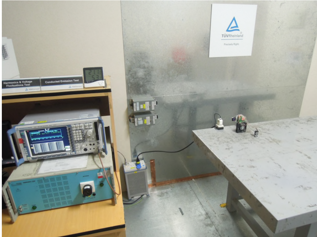
Photograph 5: Set-up for Spurious Emissions, AC Mains (Back View)
