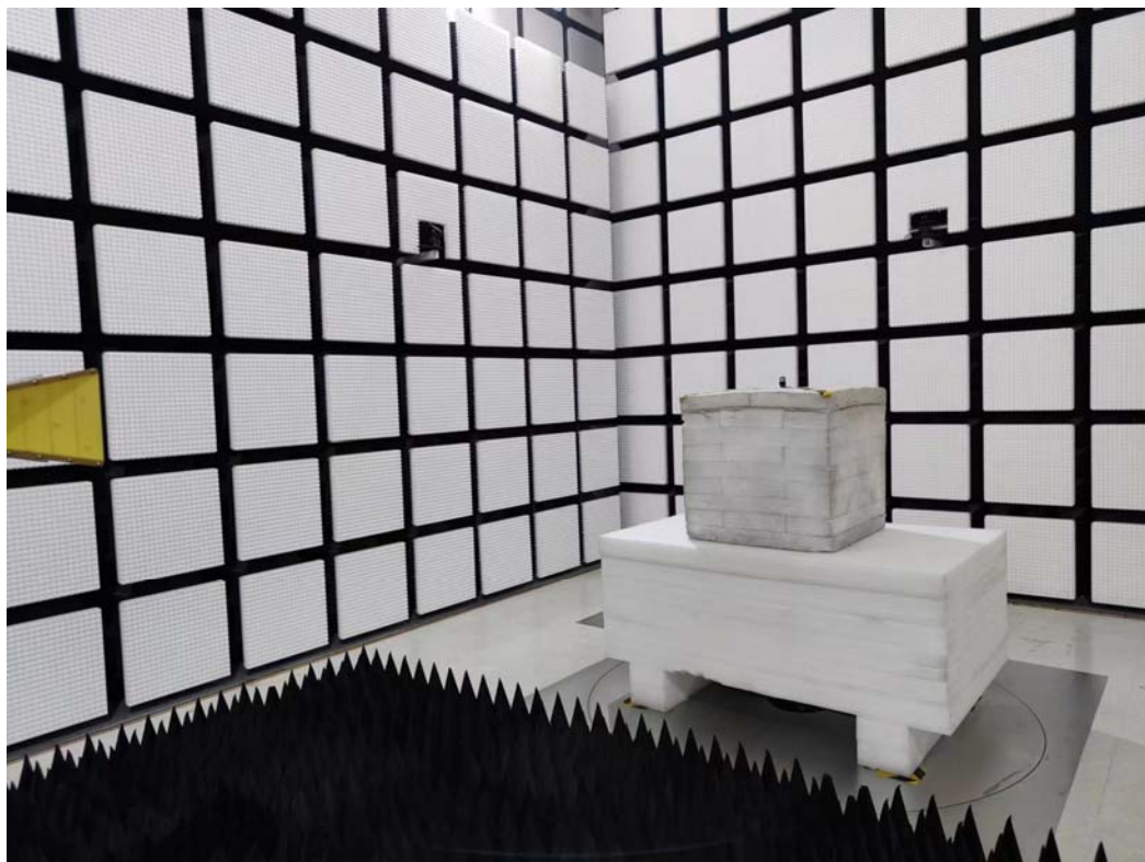
Radiated Emission Above 1GHz View
