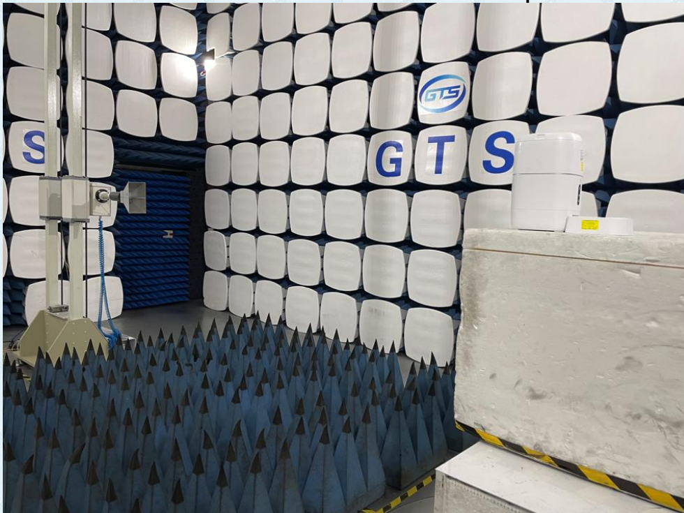
Radiated Emission Above 1GHz Test Setup
