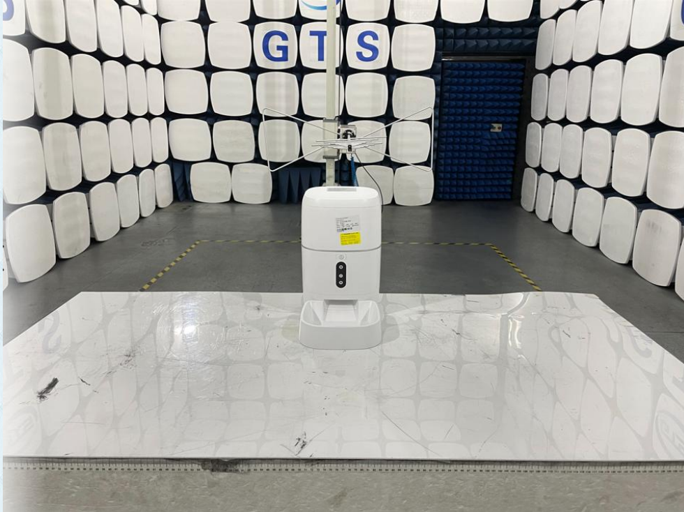
Radiated Emission Above 1GHz Test Setup
