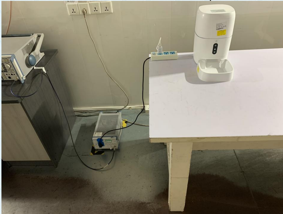
Conducted Emission Test Setup
