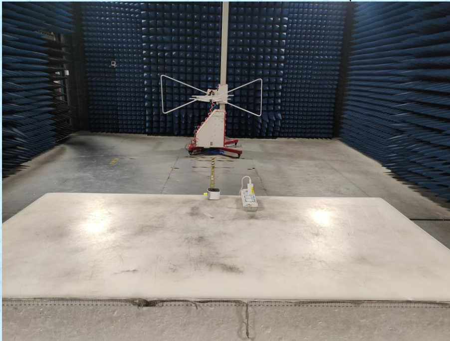
Radiated Emission Below 1GHz Test Setup
