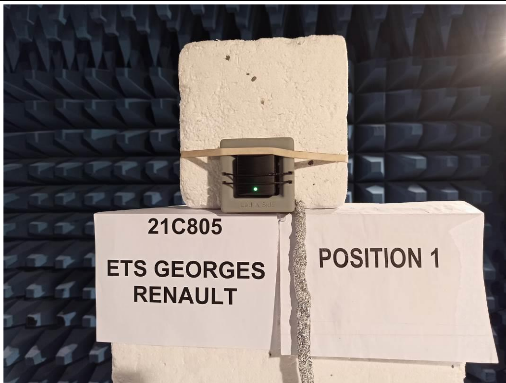
TEST SETUP PHOTO(S) - RADIATED MEASUREMENT / POSITION 1 / >GHz
