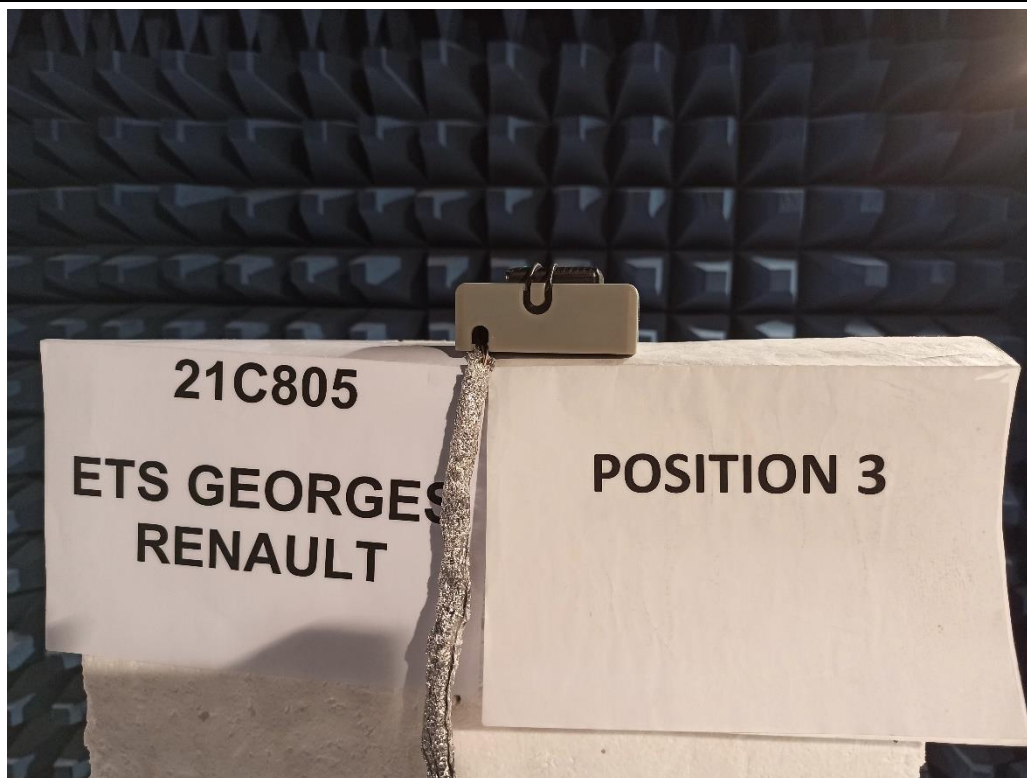
TEST SETUP PHOTO(S) - RADIATED MEASUREMENT / POSITION 3 / >GHZ
