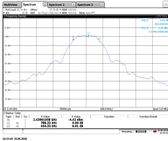
Figure 7.3.2-3: 6dB Bandwidth Mid Channel
