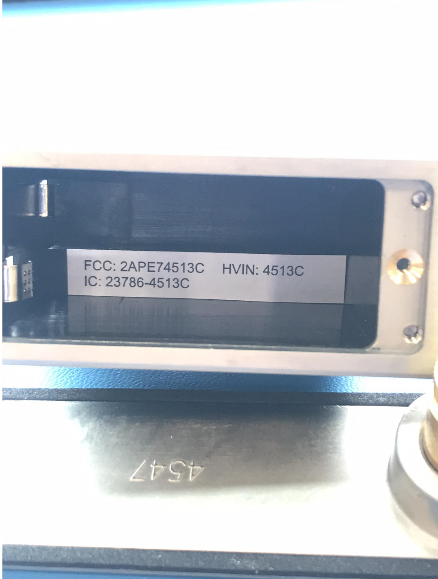
Figure 18 - Example of Label Inside Battery Compartment
