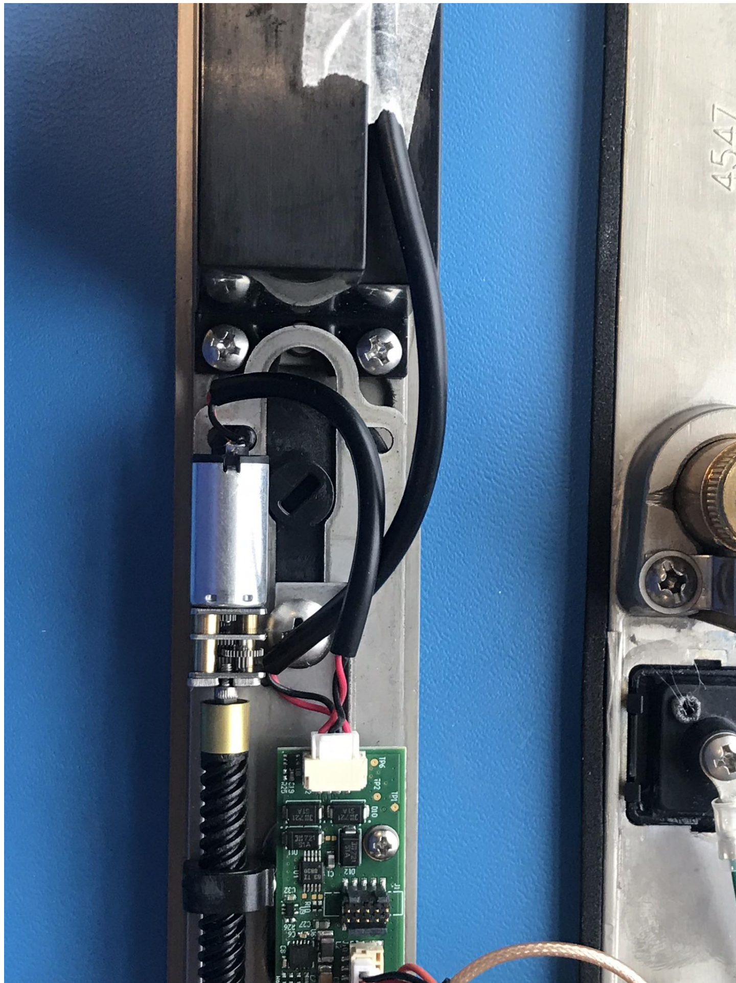
Figure 14 - Battery and Motor Connection
