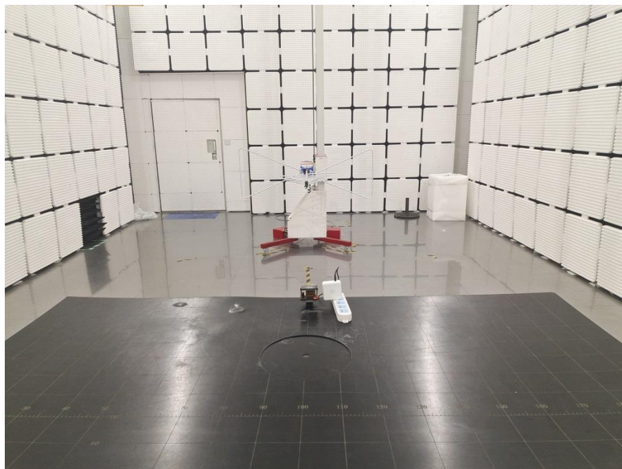
Radiated Emission (30MHz-1GHz)
