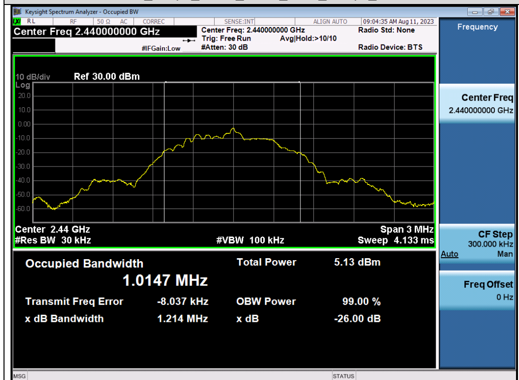
Test_Graph_LE1M_ANT1_2440_1Mbps_OBW
