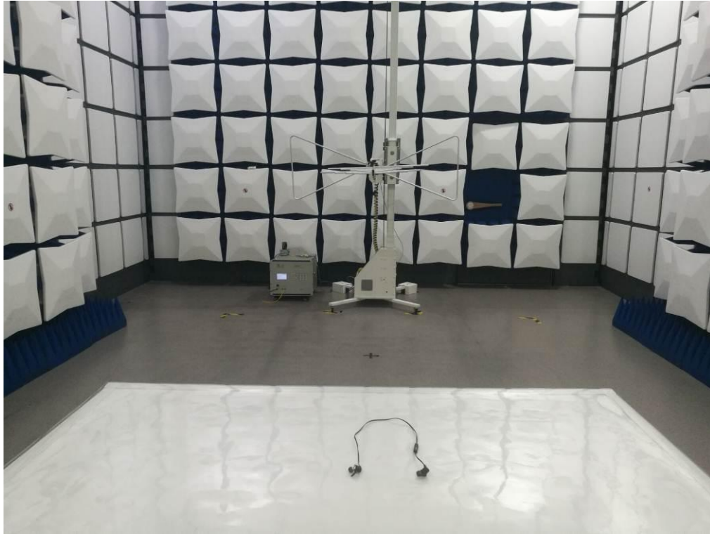
FCC RADIATED EMISSION TEST SETUP
