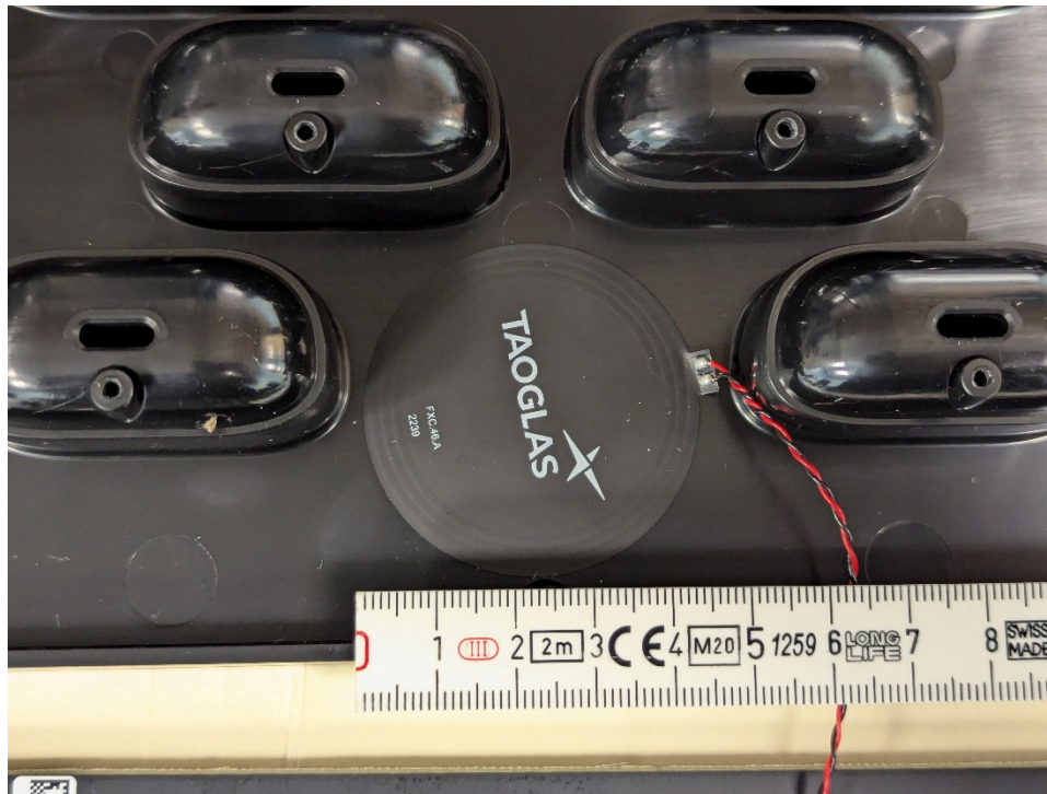
NFC Antenna mounted in Enclosure
