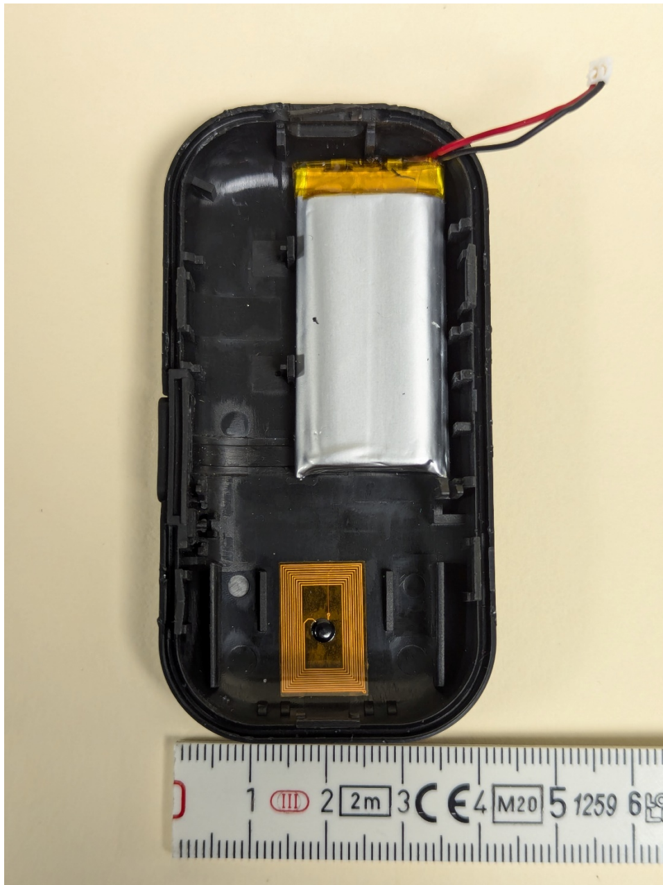
Bottom of Enclosure with PCB's and GPS Antenna Removed
