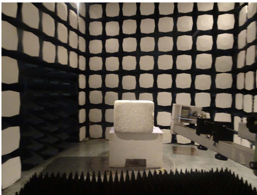
Picture 1: Radiated Spurious Emissions Test setup
