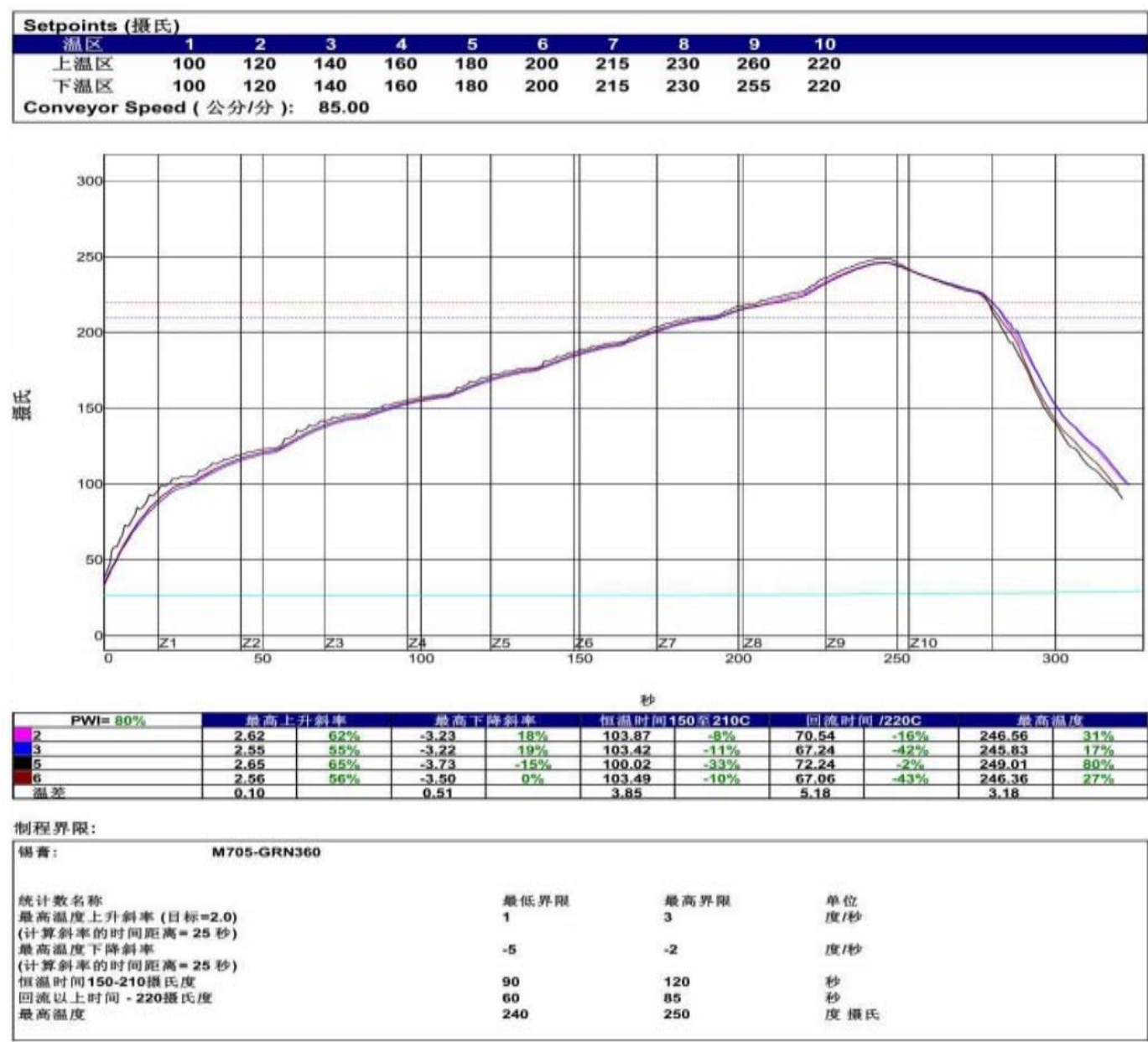
Figure 34 Reflow soldering temperature profile
