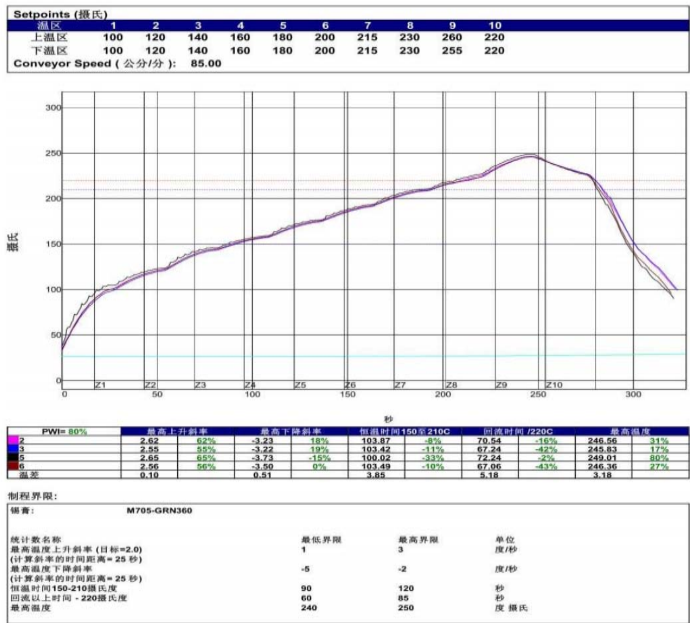
Figure 34 Reflow soldering temperature profile
