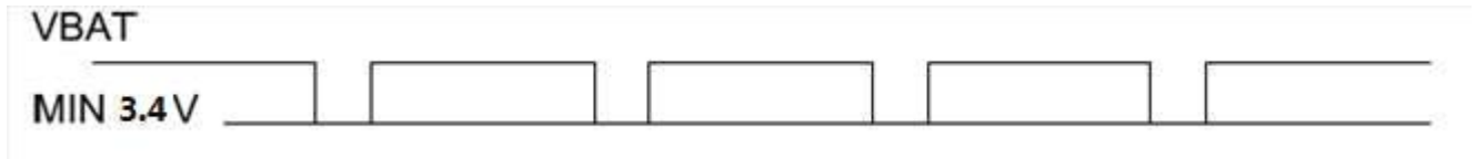
Figure 4.4 : VBAT lowest voltage drop
