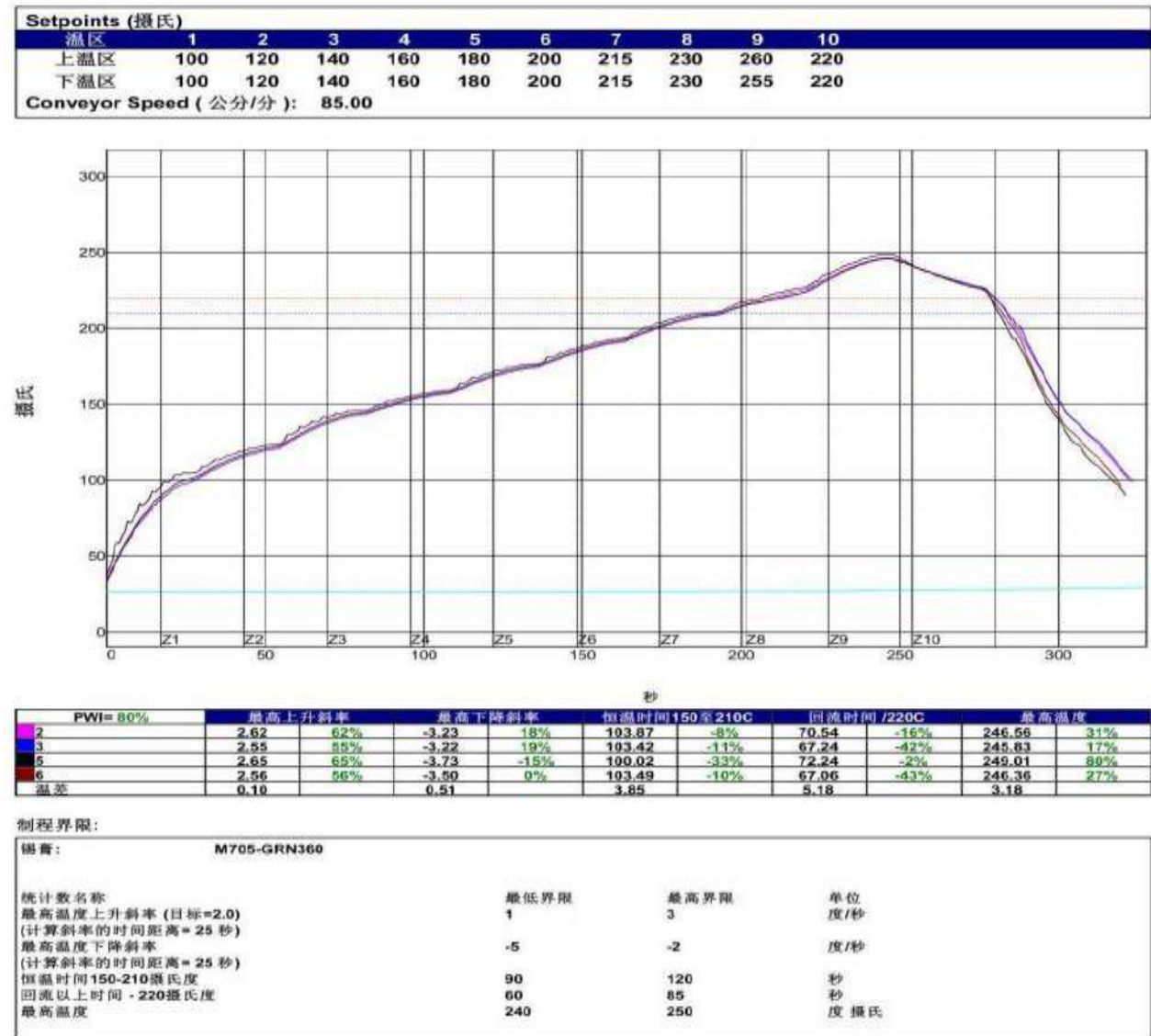
Figure 35 Reflow temperature curve
