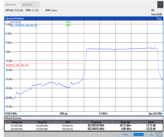
1-N5-PC3-15-10-L-3-DFT-PI2BPSK-Outer_Full-50 @0-Ant0-1-seegraph-PASS-see graph
