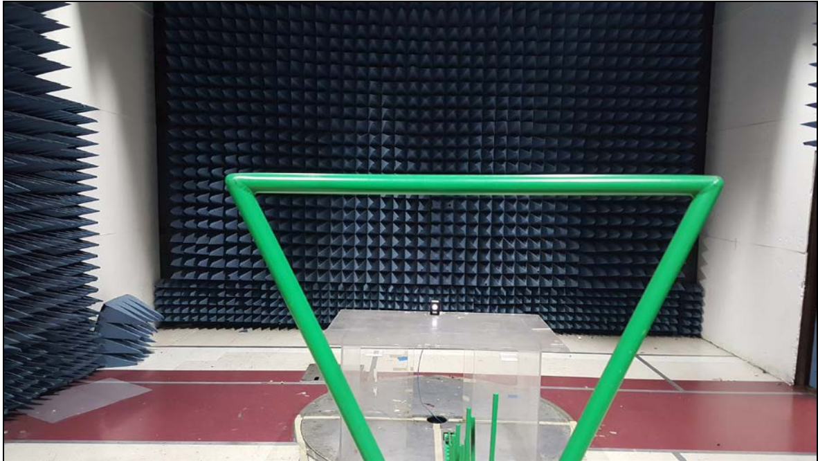
Photograph 4. Spurious Emissions, Test Setup, 30 MHz – 1 GHz
