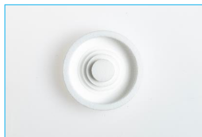
Figure 2.5. FZP lens diameter 36.3 mm and height 7.8 mm
