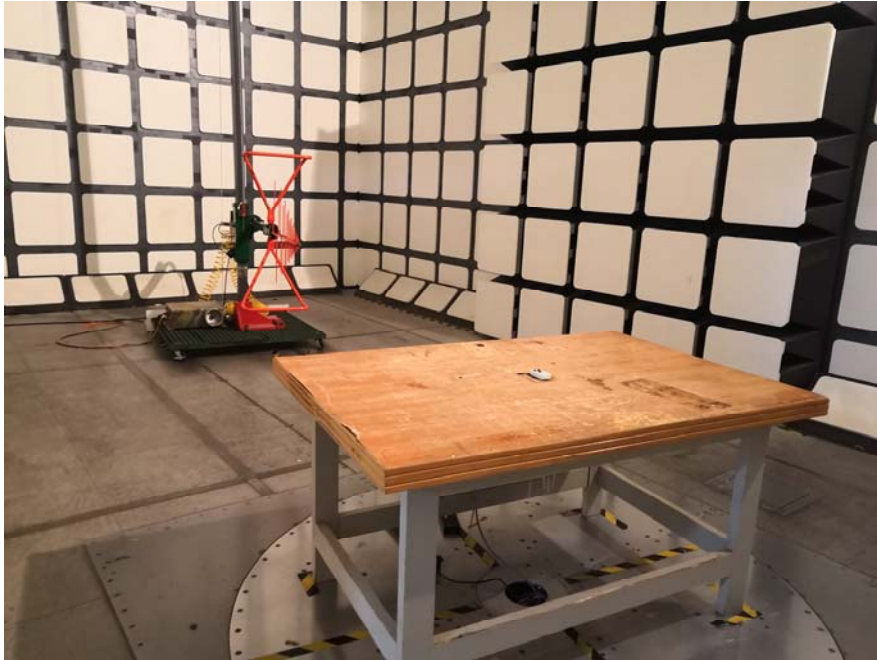
Radiated Emissions View (Below 1 GHz)
