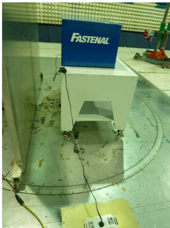
AC Mains Line-Conducted Disturbance Setup Photograph
