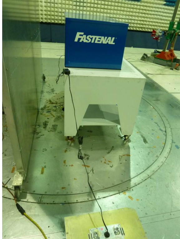
AC Mains Line-Conducted Disturbance Setup Photograph
