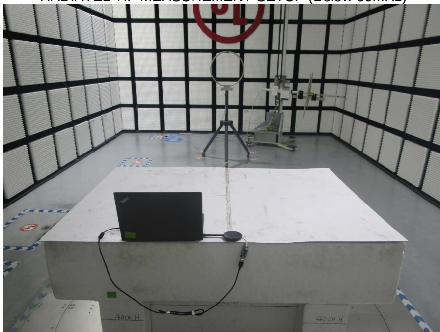
RADIATED RF MEASUREMENT SETUP (Below 30MHz)
