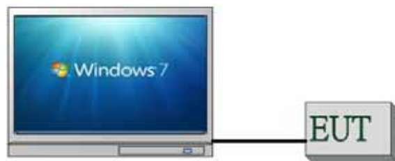
Fig. 2-3 Conducted (Antenna Port) Emission Configuration
