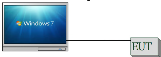
Fig. 2-1 Conducted (Antenna Port) Emission Configuration
