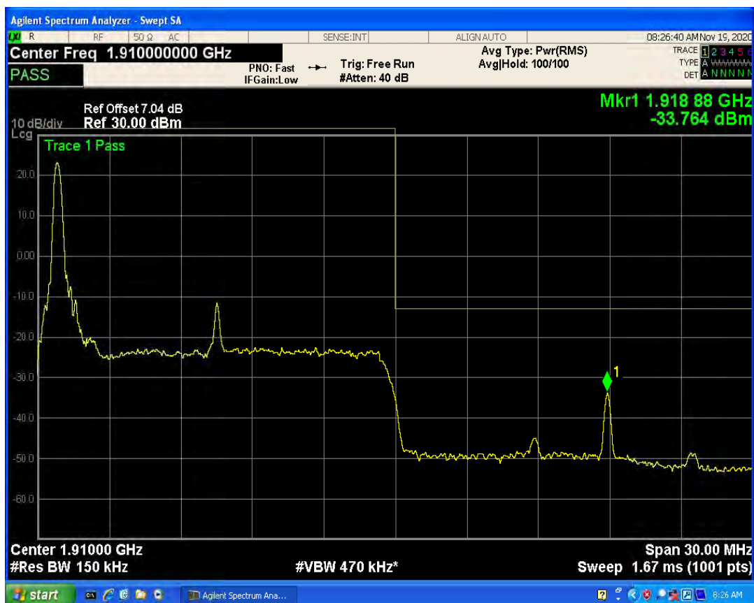
LTE Band2 QPSK BW=15MHz Channel=19125 RB Size=1 Position=#Max
