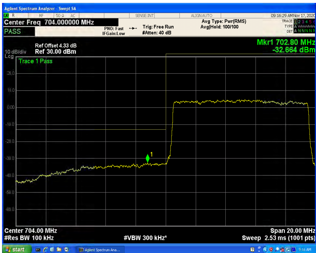
LTE Band17 QPSK BW=10MHz Channel=23800 RB Size=1 Position=#0
