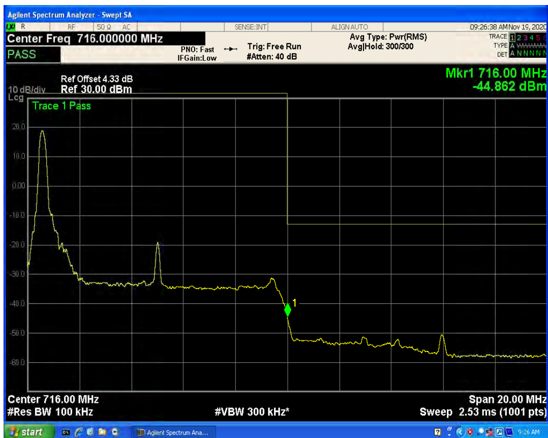
LTE Band12 QAM16 BW=10MHz Channel=23130 RB Size=1 Position=#Max
