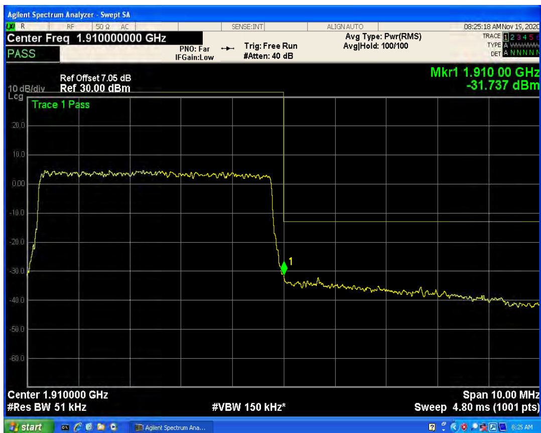
LTE Band2 QPSK BW=10MHz Channel=18650 RB Size=1 Position=#0
