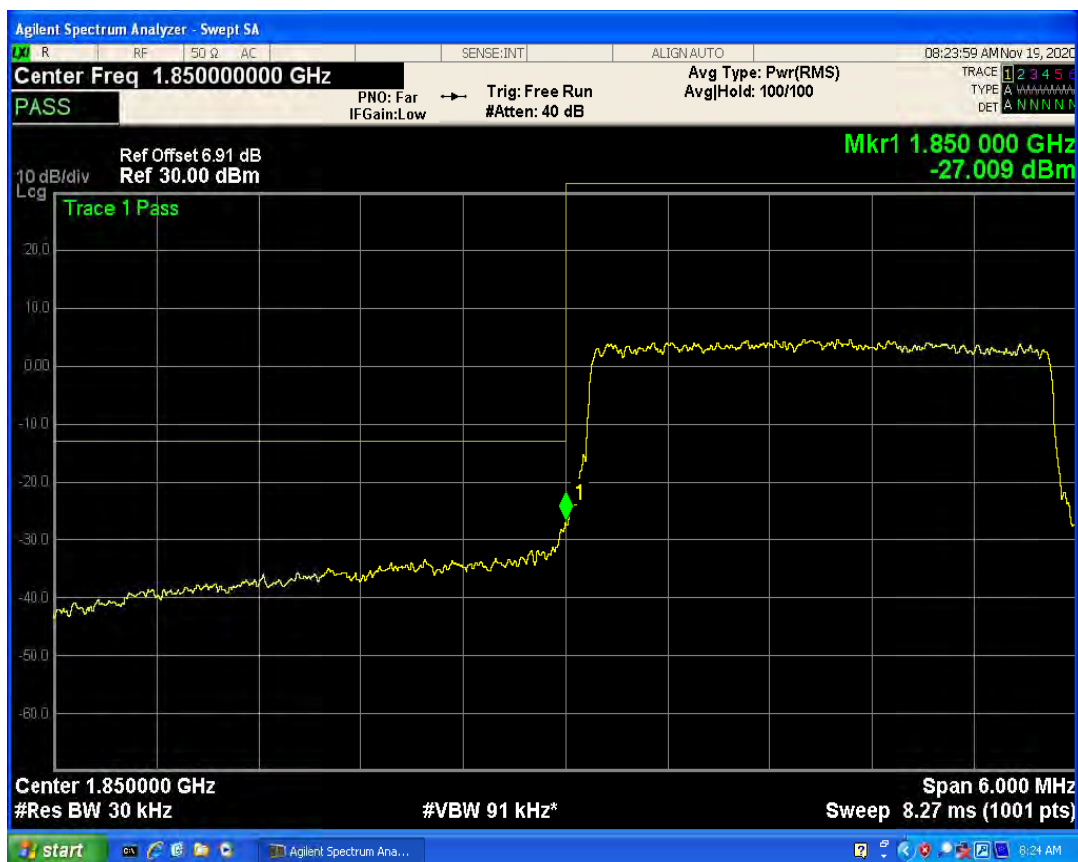
LTE Band2 QPSK BW=3MHz Channel=19185 RB Size=1 Position=#0
