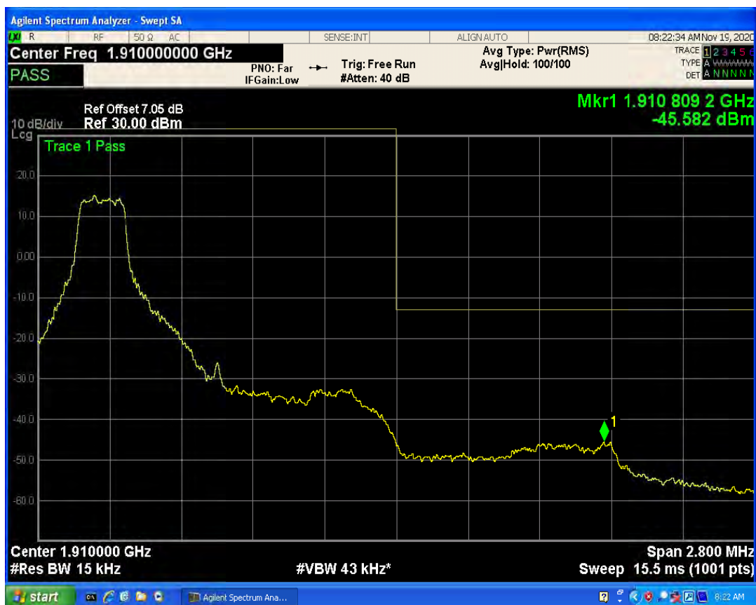
LTE Band2 QPSK BW=1.4MHz Channel=19193 RB Size=1 Position=#Max
