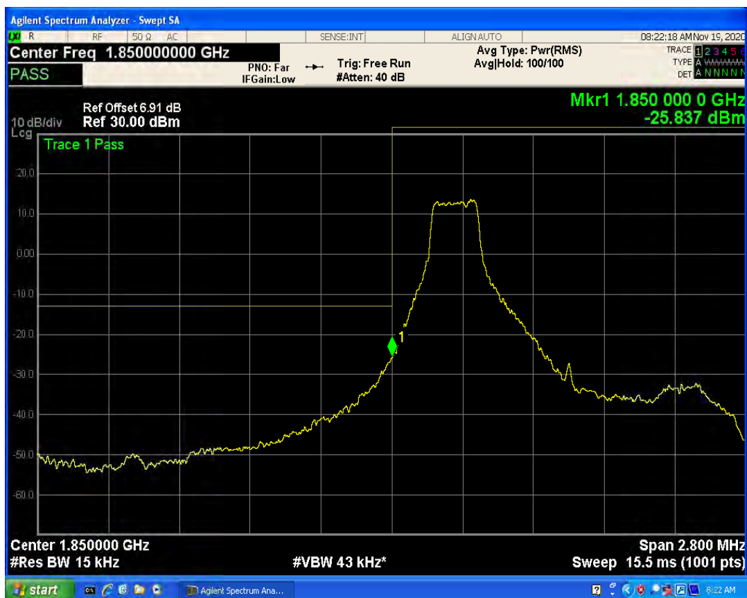
LTE Band2 QPSK BW=1.4MHz Channel=18607 RB Size=6 Position=#0
