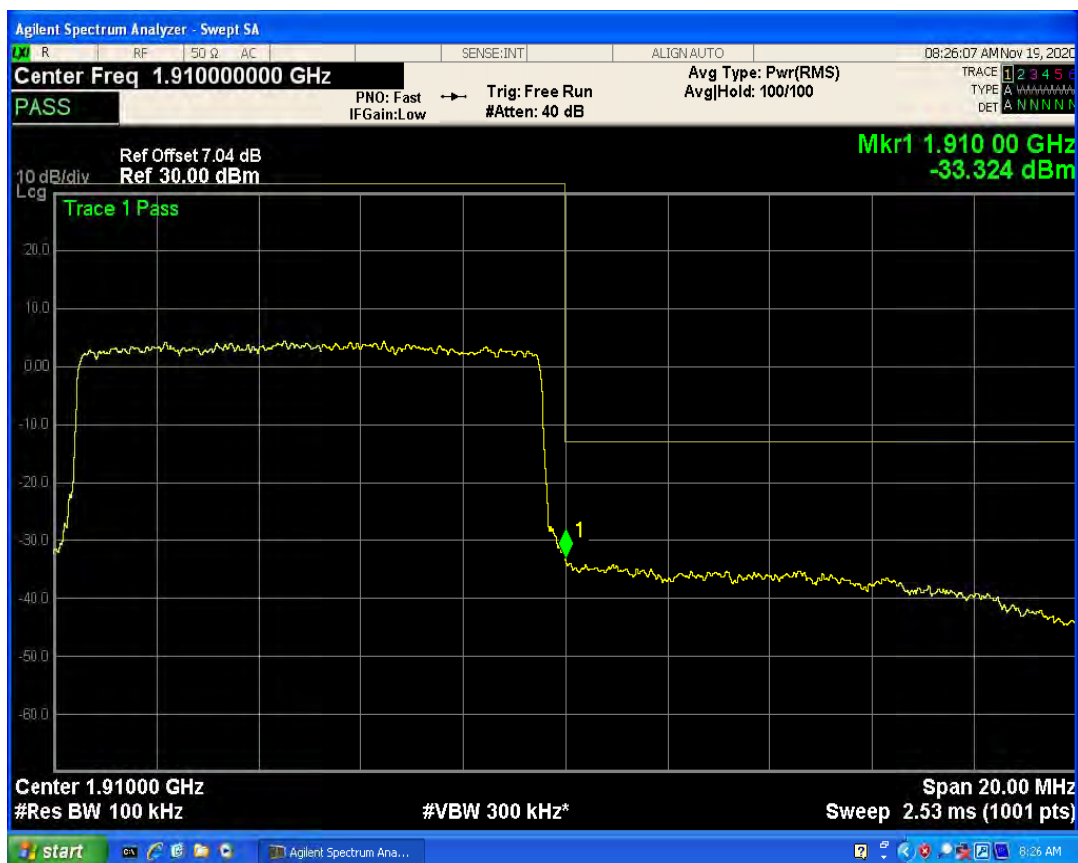
LTE Band2 QAM16 BW=10MHz Channel=19150 RB Size=1 Position=#Max
