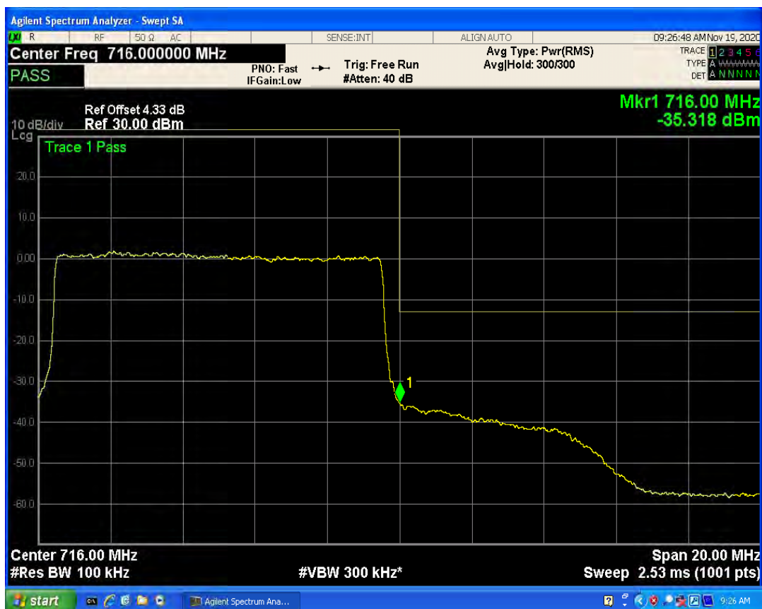
LTE Band12 QPSK BW=3MHz Channel=23025 RB Size=1 Position=#Max
