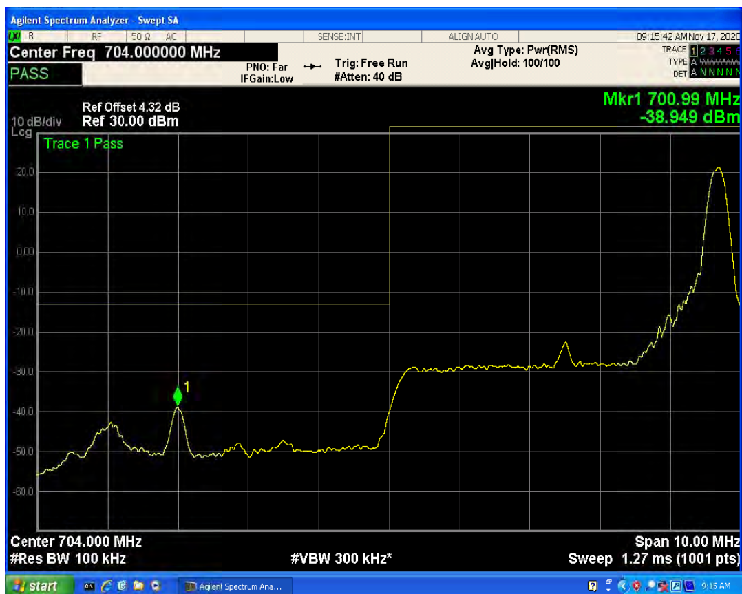
LTE Band17 QAM16 BW=5MHz Channel=23755 RB Size=25 Position=#0
