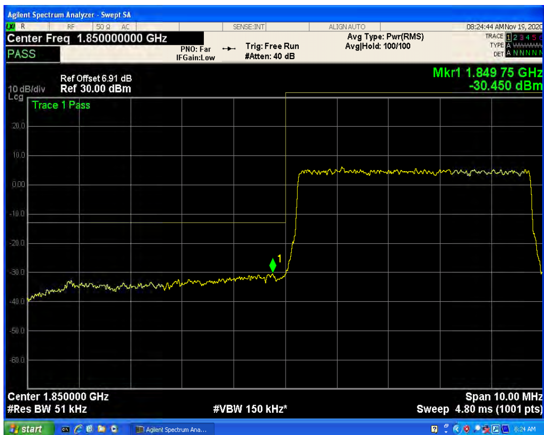
LTE Band2 QAM16 BW=5MHz Channel=18625 RB Size=1 Position=#Max
