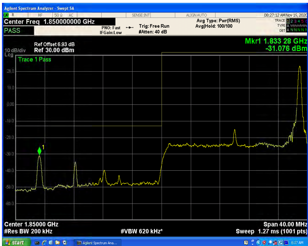
LTE Band2 QPSK BW=20MHz Channel=18700 RB Size=100 Position=#0
