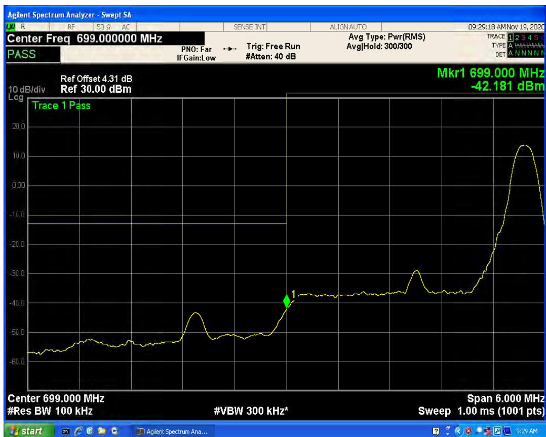
LTE Band12 QPSK BW=3MHz Channel=23165 RB Size=1 Position=#0
