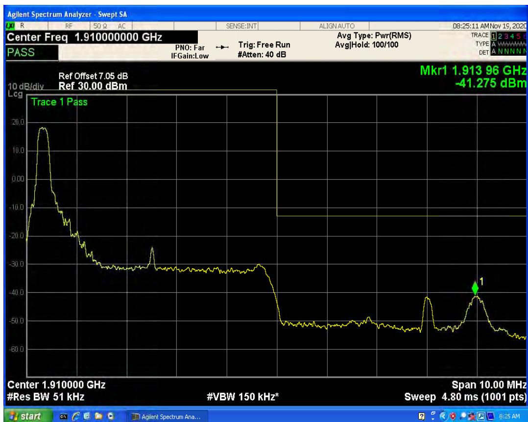
LTE Band2 QAM16 BW=5MHz Channel=19175 RB Size=1 Position=#Max
