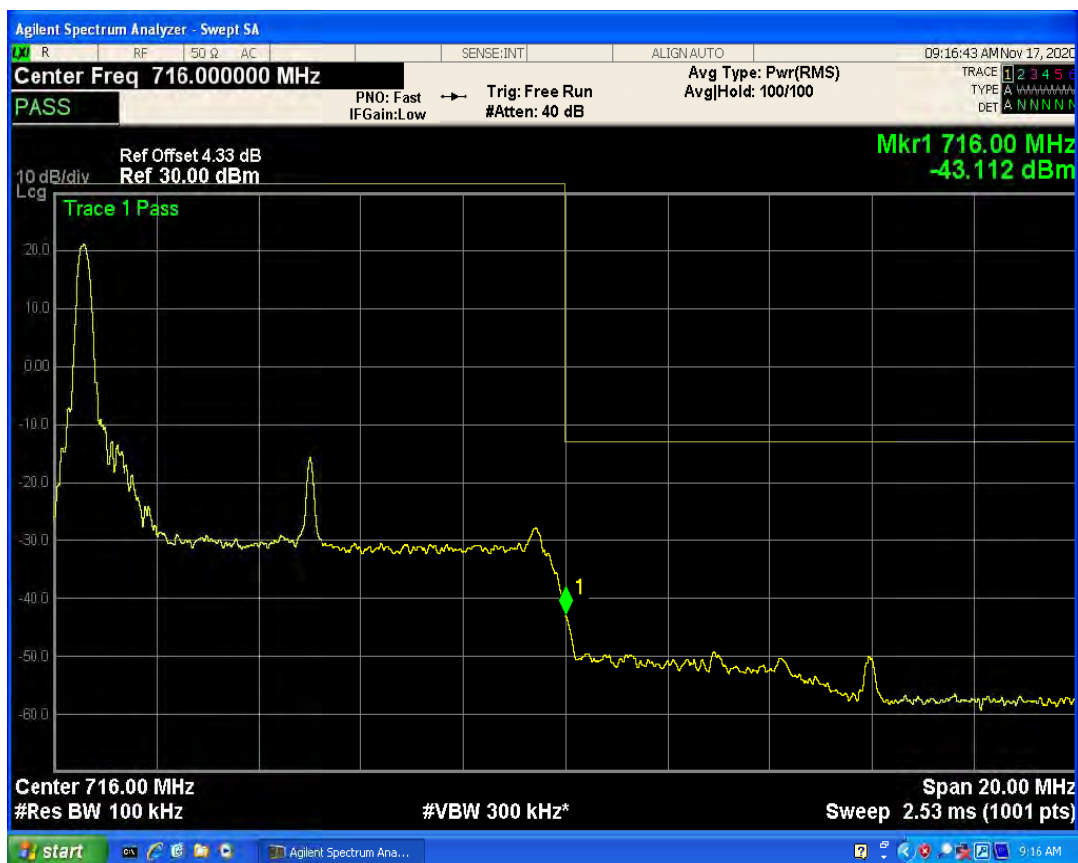
LTE Band17 QAM16 BW=10MHz Channel=23800 RB Size=50 Position=#0
