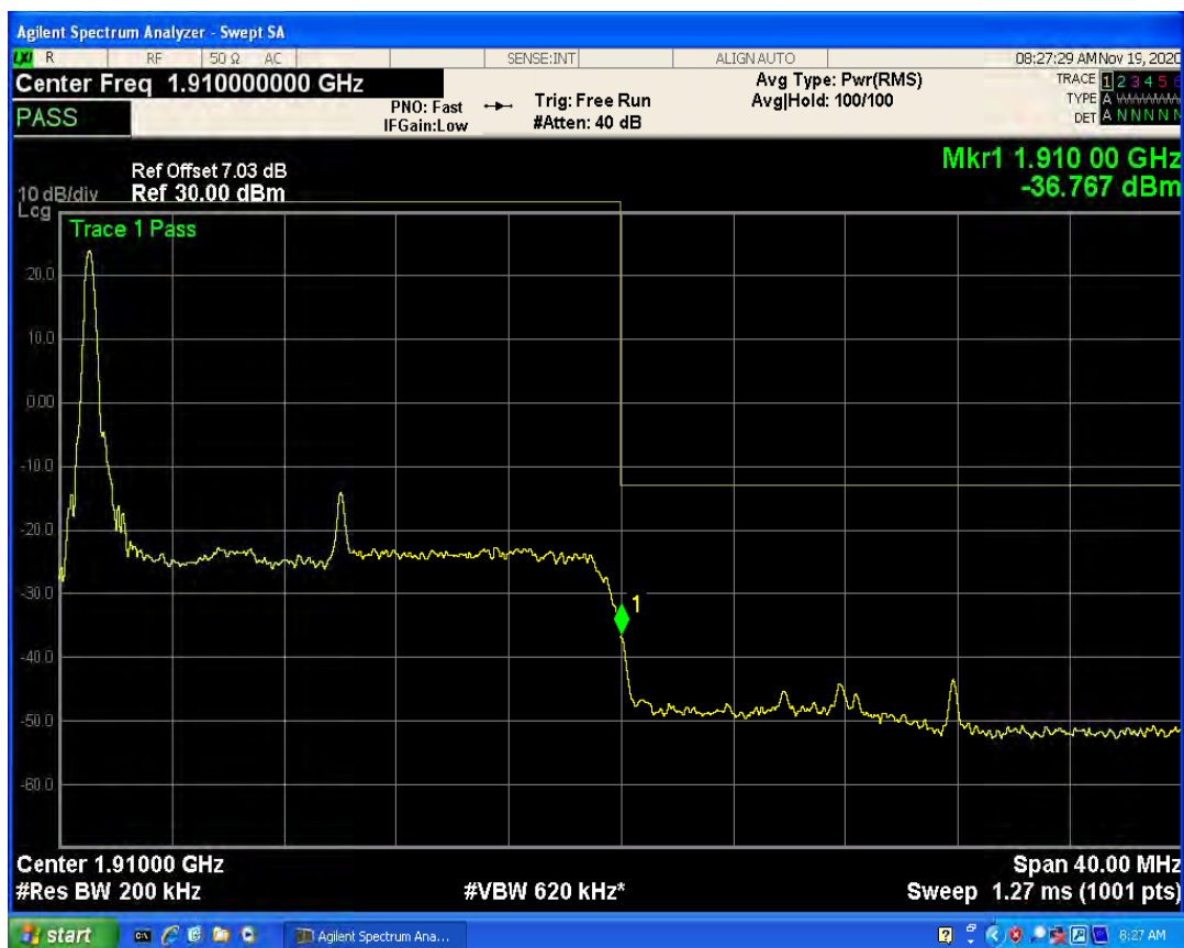
LTE Band2 QPSK BW=20MHz Channel=19100 RB Size=1 Position=#Max
