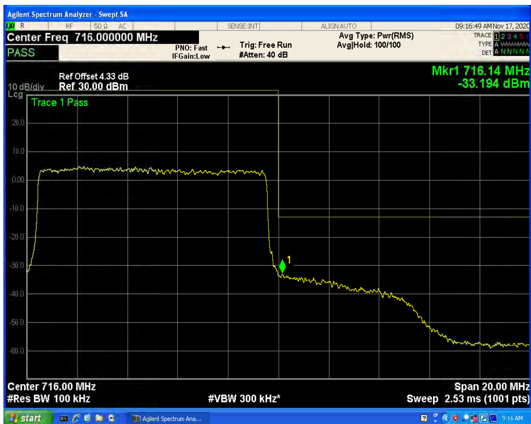
LTE Band2 QPSK BW=1.4MHz Channel=18607 RB Size=1 Position=#0
