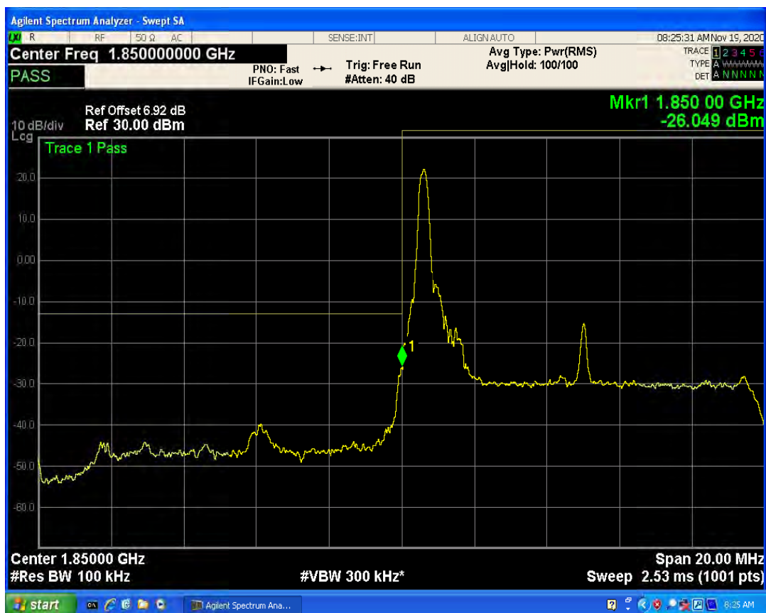
LTE Band2 QPSK BW=10MHz Channel=18650 RB Size=1 Position=#Max
