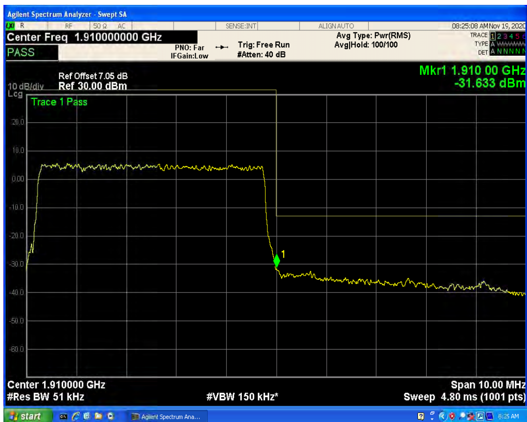
LTE Band2 QAM16 BW=5MHz Channel=19175 RB Size=1 Position=#0
