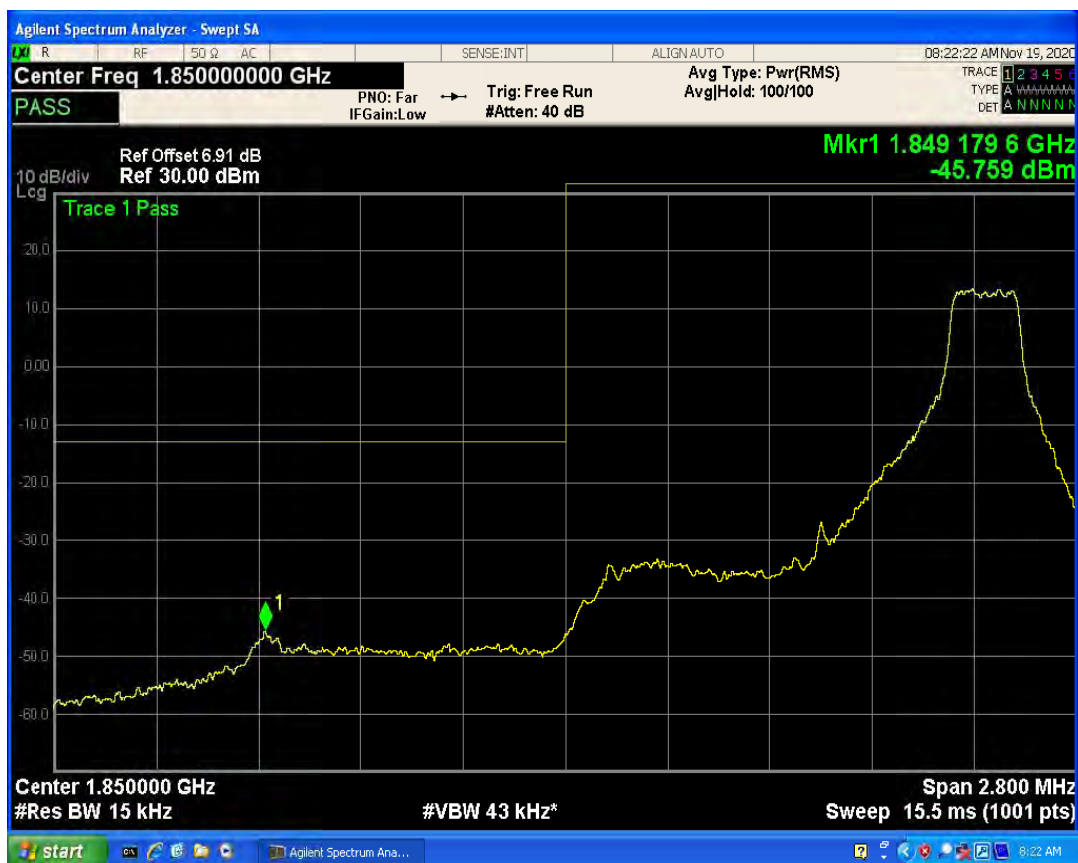
LTE Band2 QAM16 BW=1.4MHz Channel=18607 RB Size=6 Position=#0
