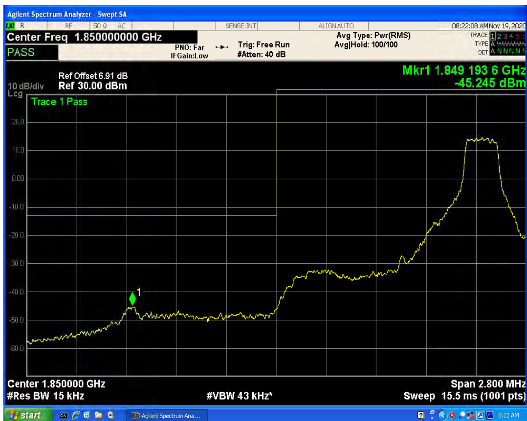
LTE Band2 QAM16 BW=1.4MHz Channel=18607 RB Size=1 Position=#0
