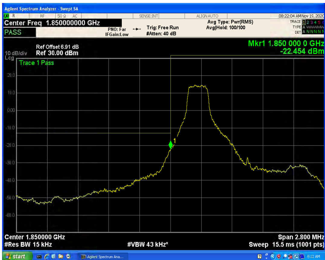
LTE Band2 QPSK BW=1.4MHz Channel=18607 RB Size=1 Position=#Max
