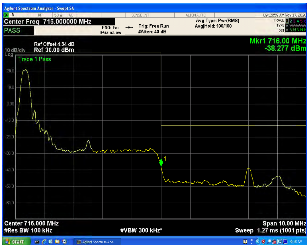
LTE Band17 QAM16 BW=5MHz Channel=23825 RB Size=1 Position=#Max
