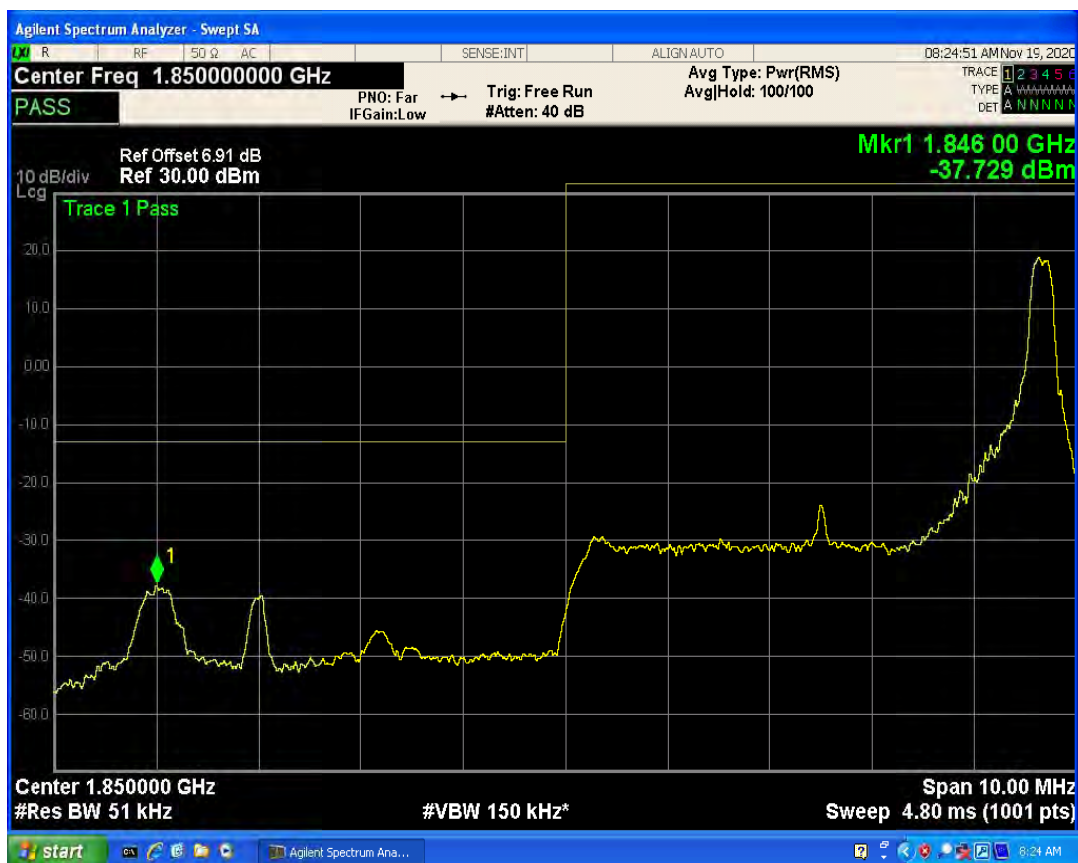
LTE Band2 QAM16 BW=5MHz Channel=18625 RB Size=25 Position=#0
