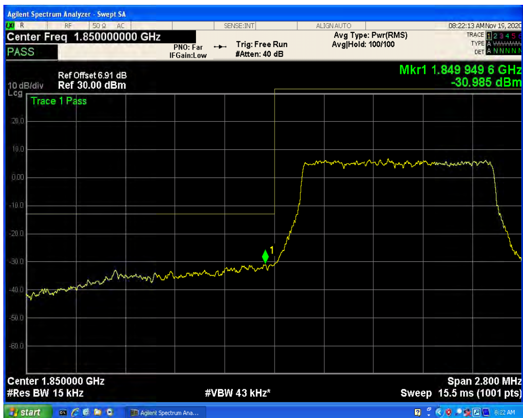
LTE Band2 QAM16 BW=1.4MHz Channel=18607 RB Size=1 Position=#Max
