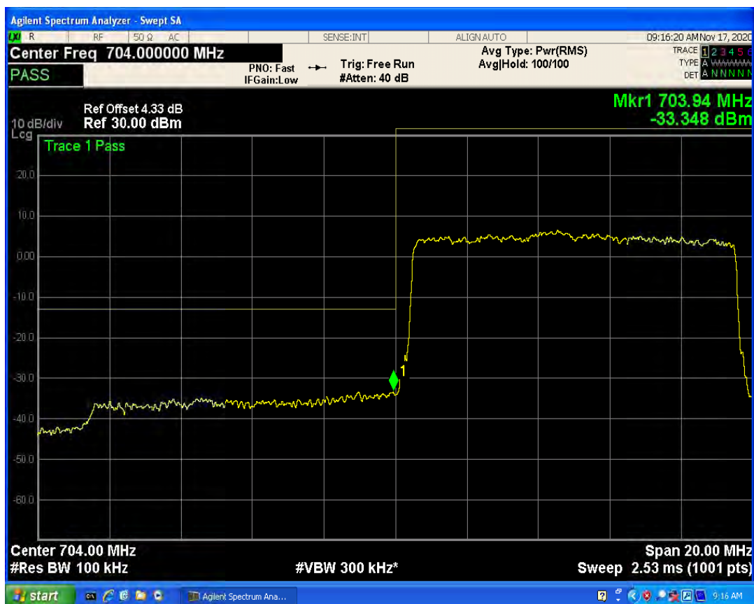
LTE Band17 QAM16 BW=10MHz Channel=23780 RB Size=1 Position=#0
