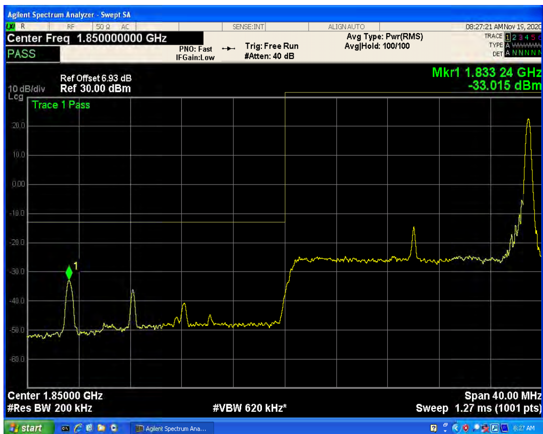
LTE Band2 QAM16 BW=20MHz Channel=18700 RB Size=100 Position=#0
