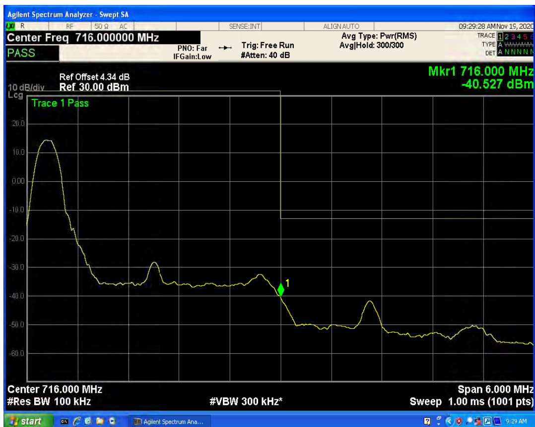
LTE Band12 QAM16 BW=3MHz Channel=23025 RB Size=15 Position=#0
