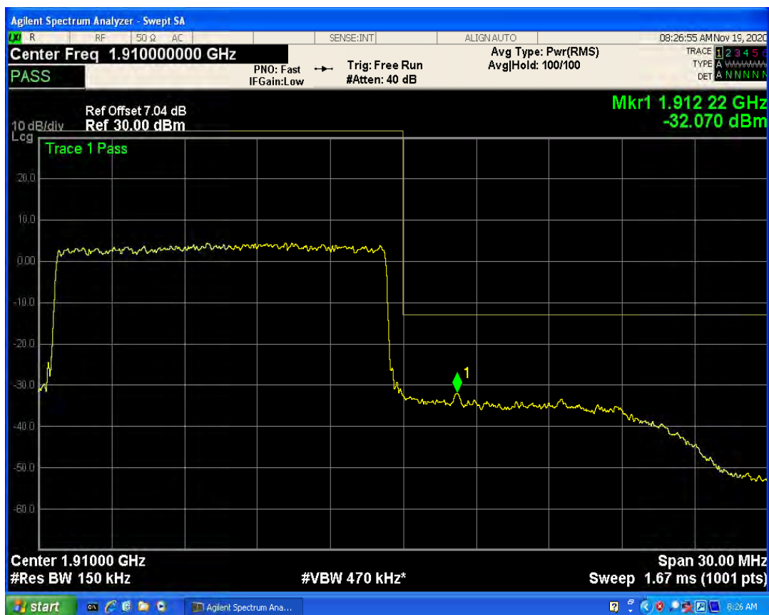
LTE Band2 QPSK BW=20MHz Channel=18700 RB Size=1 Position=#0
