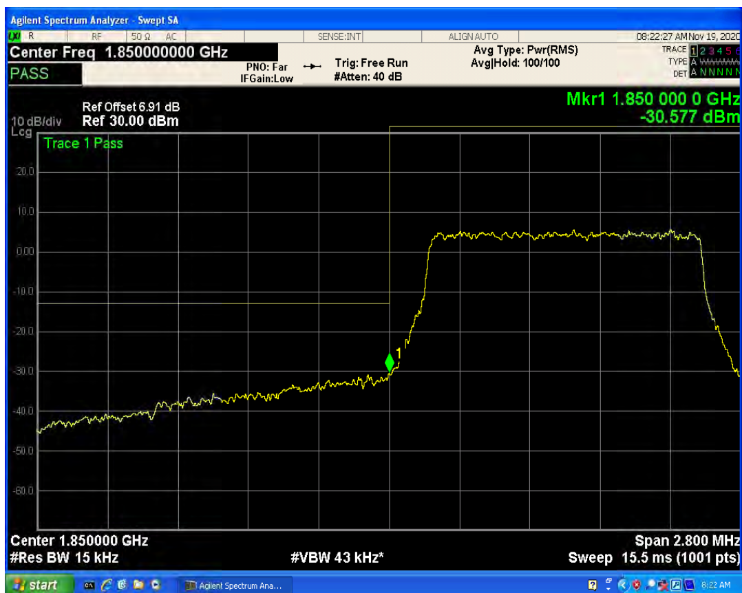
LTE Band2 QPSK BW=1.4MHz Channel=19193 RB Size=1 Position=#0
