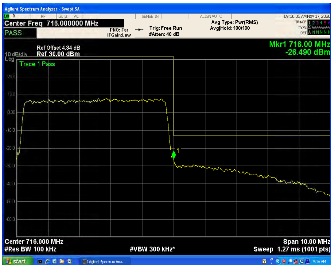
LTE Band17 QPSK BW=10MHz Channel=23780 RB Size=1 Position=#Max
