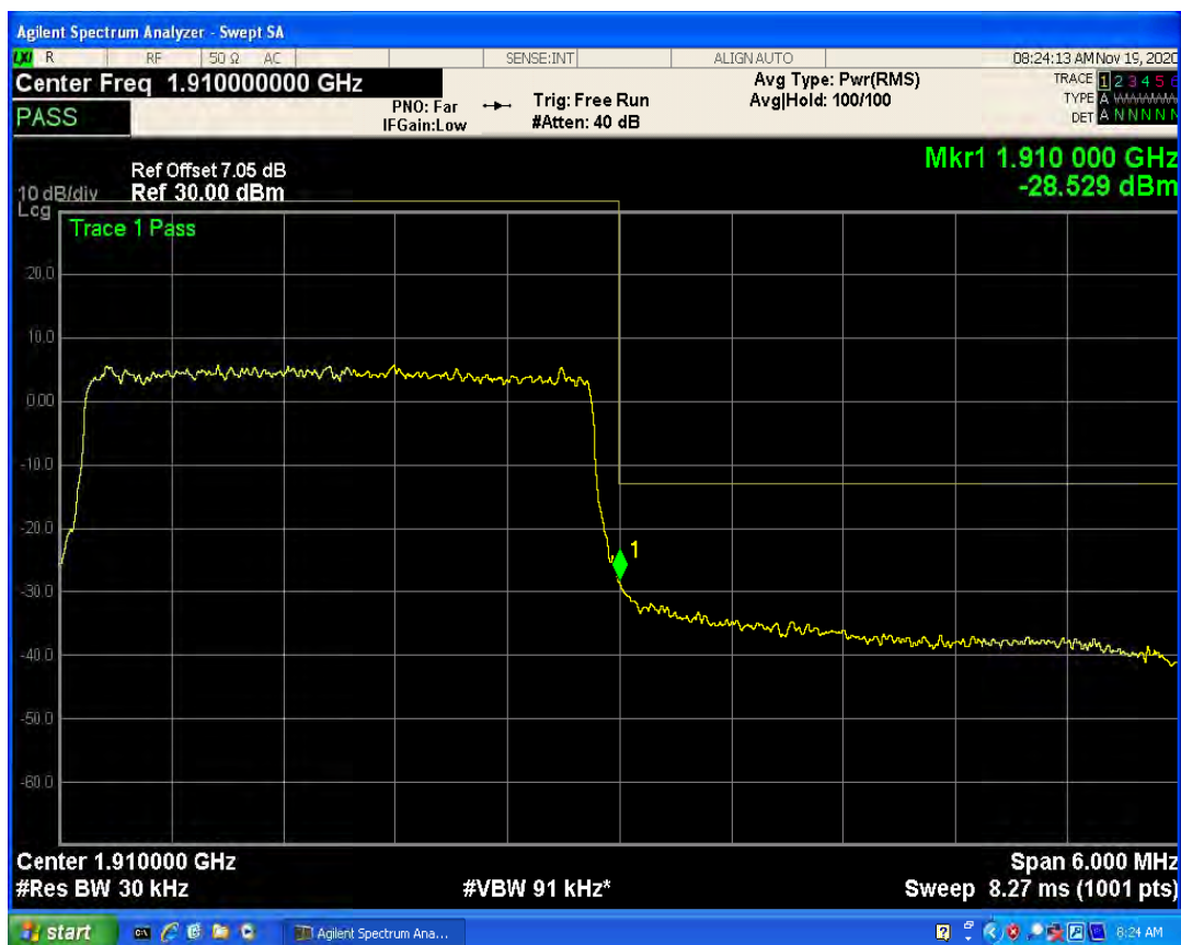
LTE Band2 QAM16 BW=3MHz Channel=19185 RB Size=1 Position=#0
