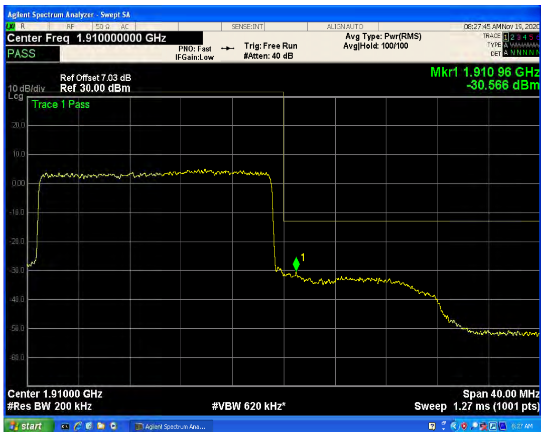
LTE Band4 QPSK BW=1.4MHz Channel=19957 RB Size=1 Position=#Max
