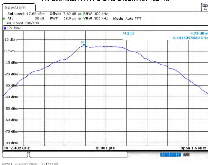
Tx. Spurious NVNT 1-DH5 2402MHz Ant1 Ref
