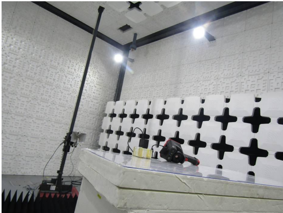
Radiated Emission (Above 1GHz)
