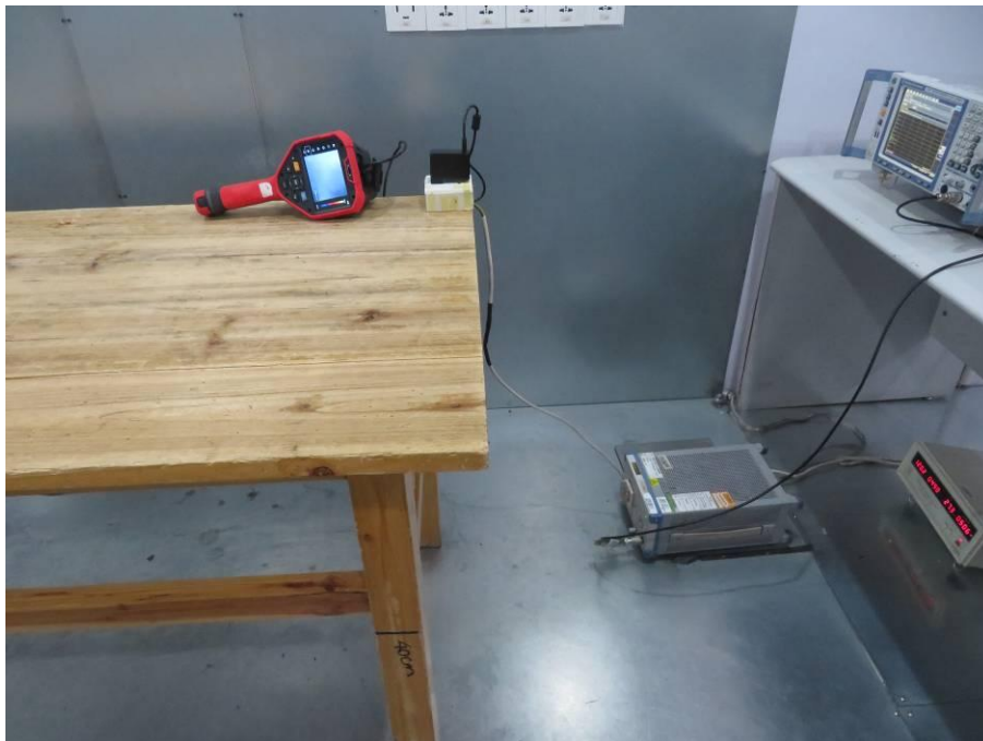
Conducted Emissions at Mains Terminals
