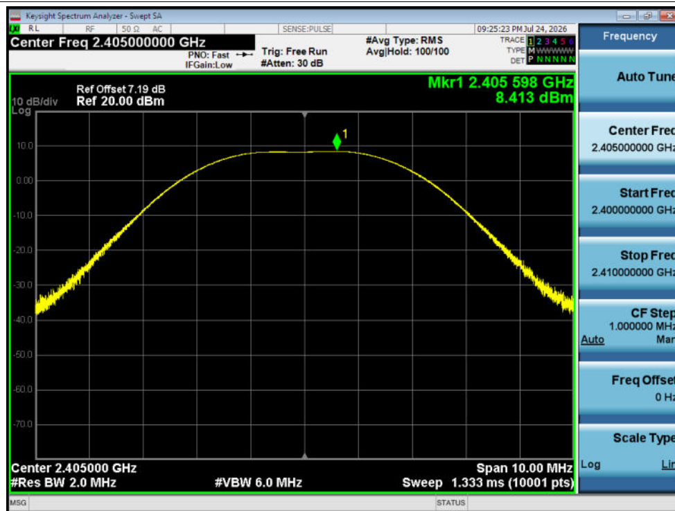
Peak Power NVNT Zigbee 2405MHz Ant1
