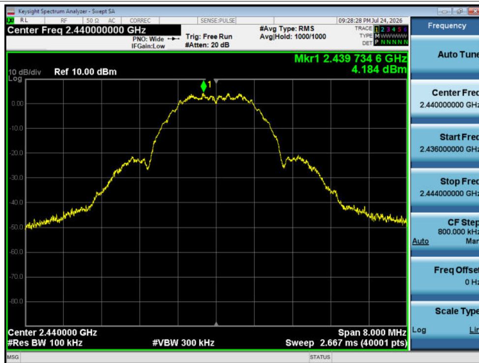
Tx. Spurious NVNT Zigbee 2440MHz Ant1 Ref
