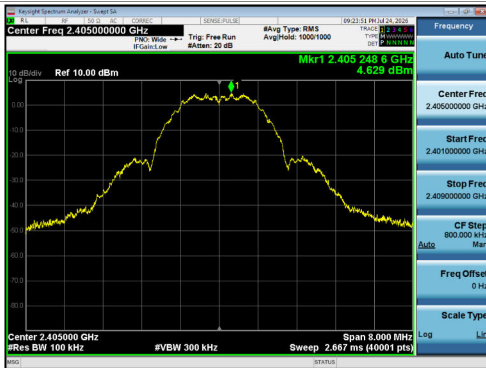
Tx. Spurious NVNT Zigbee 2405MHz Ant1 Ref
