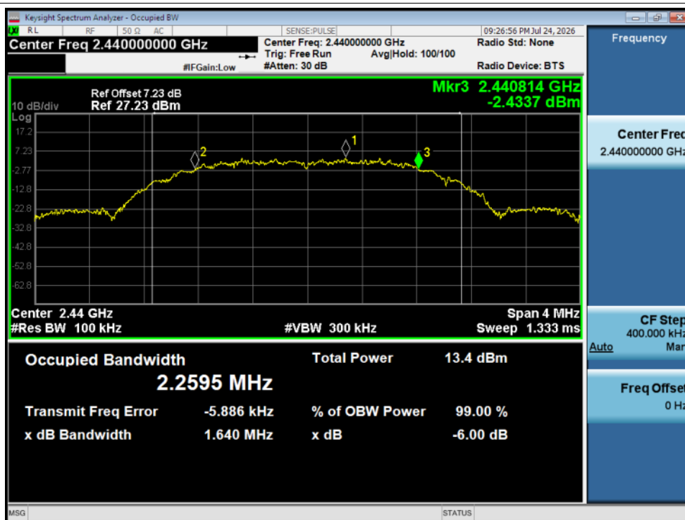
-6dB Bandwidth NVNT Zigbee 2440MHz Ant1
