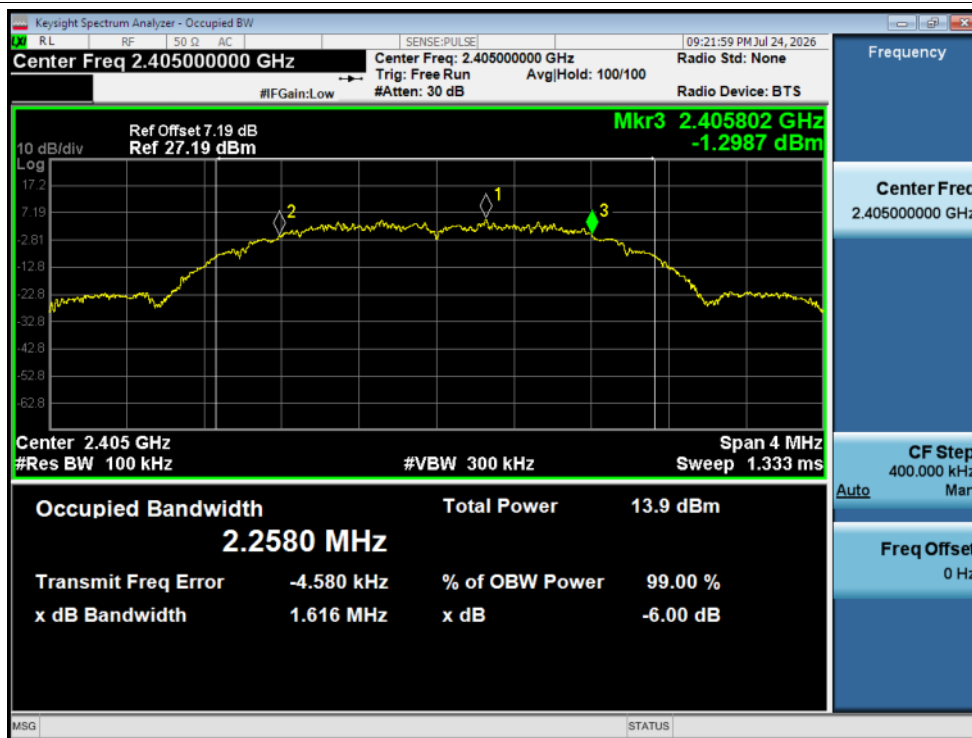
-6dB Bandwidth NVNT Zigbee 2405MHz Ant1
