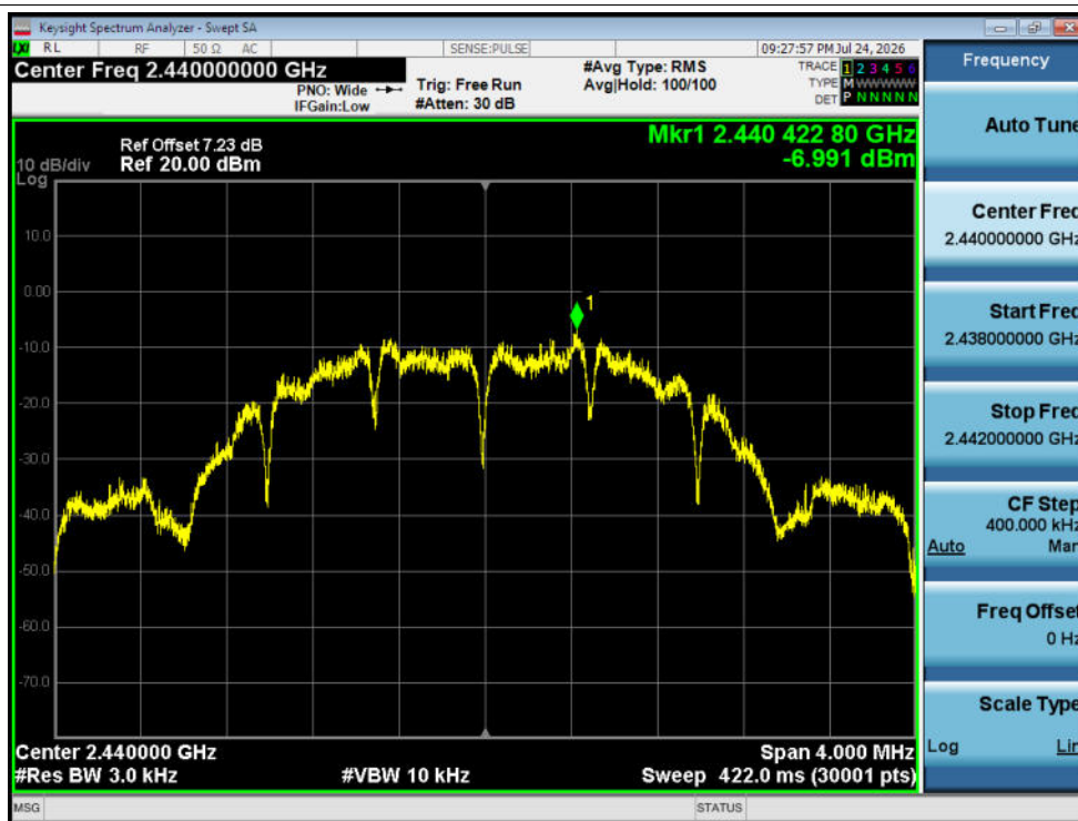
PSD NVNT Zigbee 2440MHz Ant1
