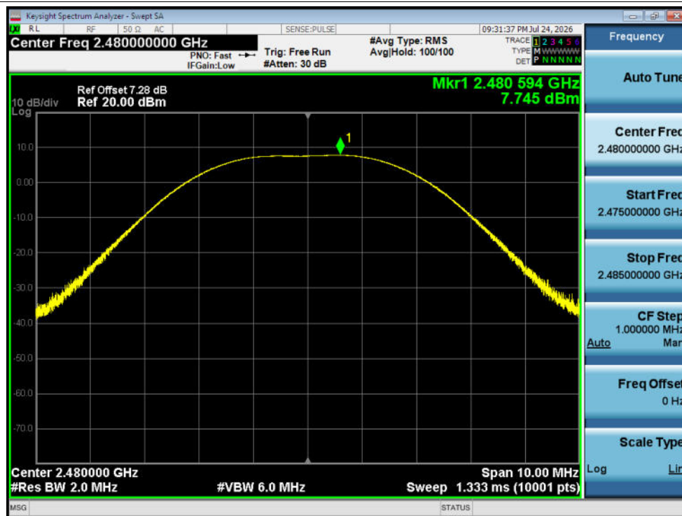
Peak Power NVNT Zigbee 2480MHz Ant1
