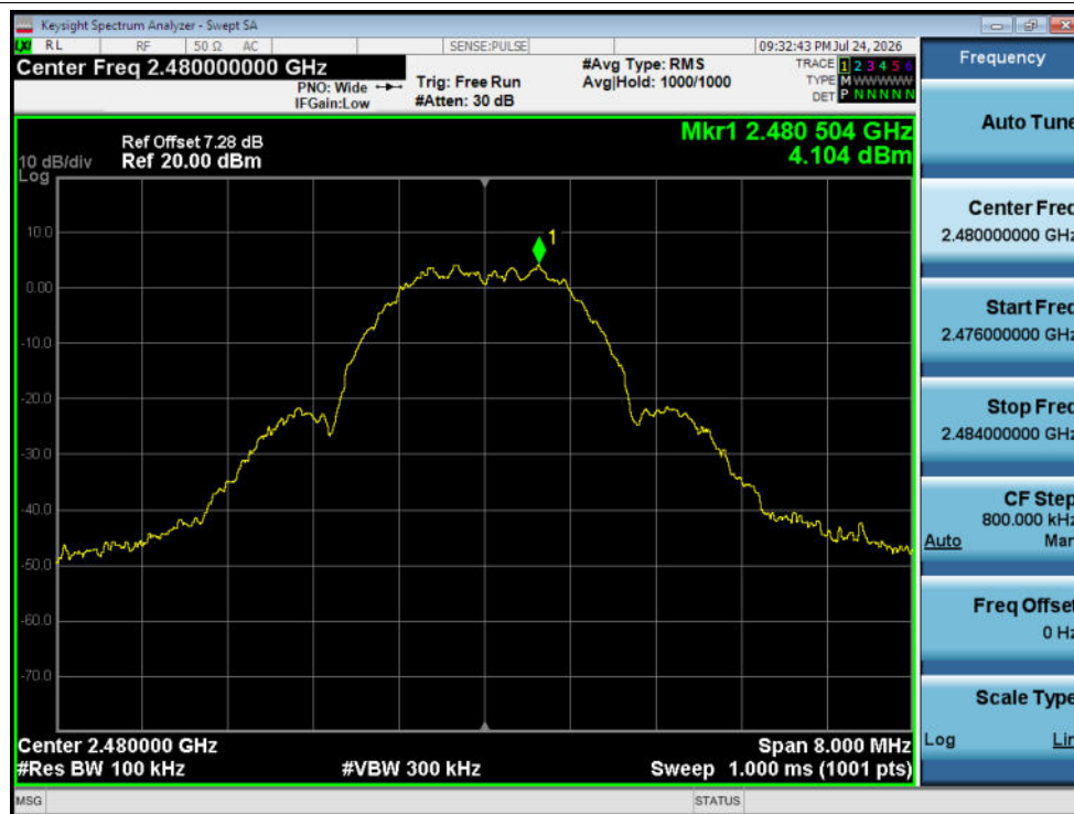
Band Edge NVNT Zigbee 2480MHz Ant1 Ref
