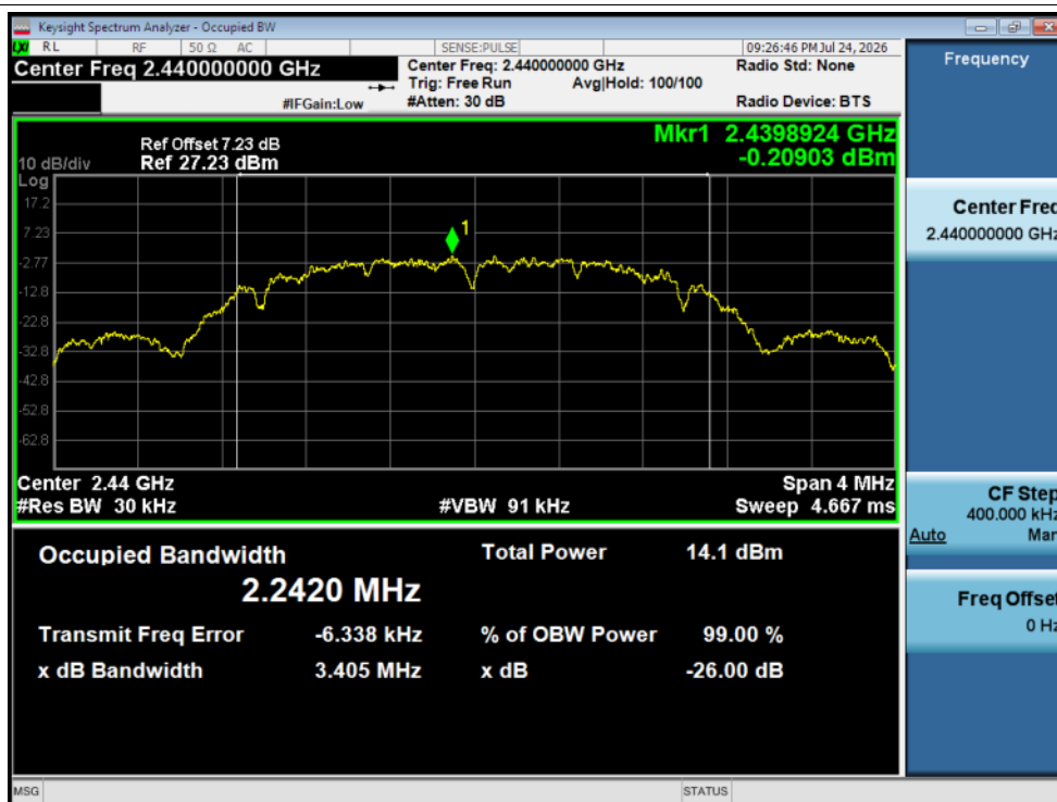
OBW NVNT Zigbee 2440MHz Ant1
