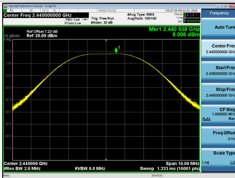
Peak Power NVNT Zigbee 2440MHz Ant1
