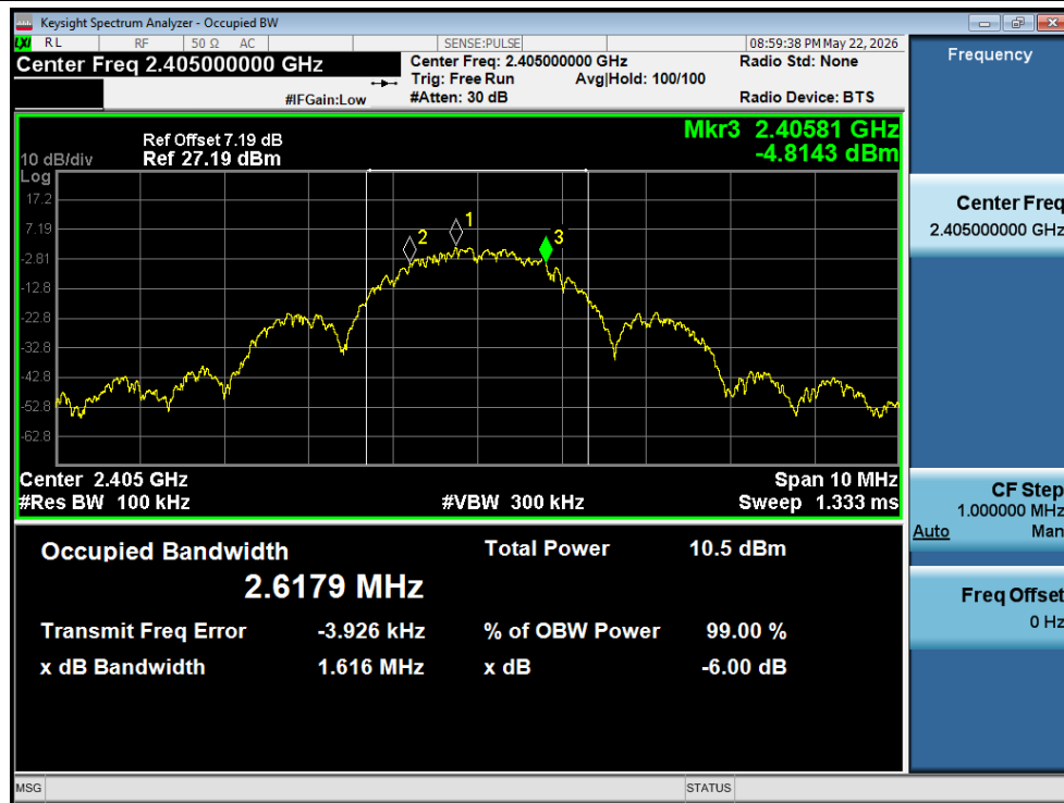
-6dB Bandwidth NVNT Zigbee 2405MHz Ant1
