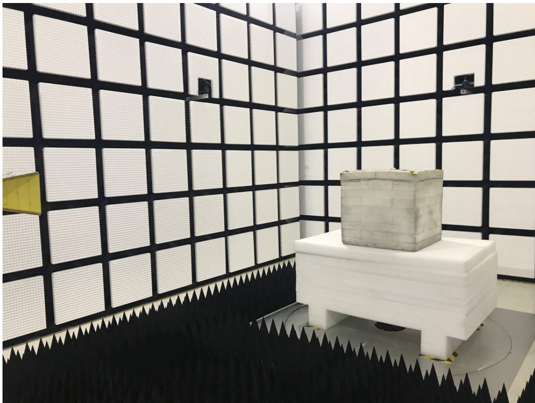
Radiated Emissions Above 1G front View
