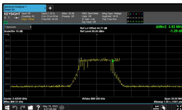
Figure 17 - LTE Full Resource Blocks 4.5 MHz BW Minimum 99% OBW
