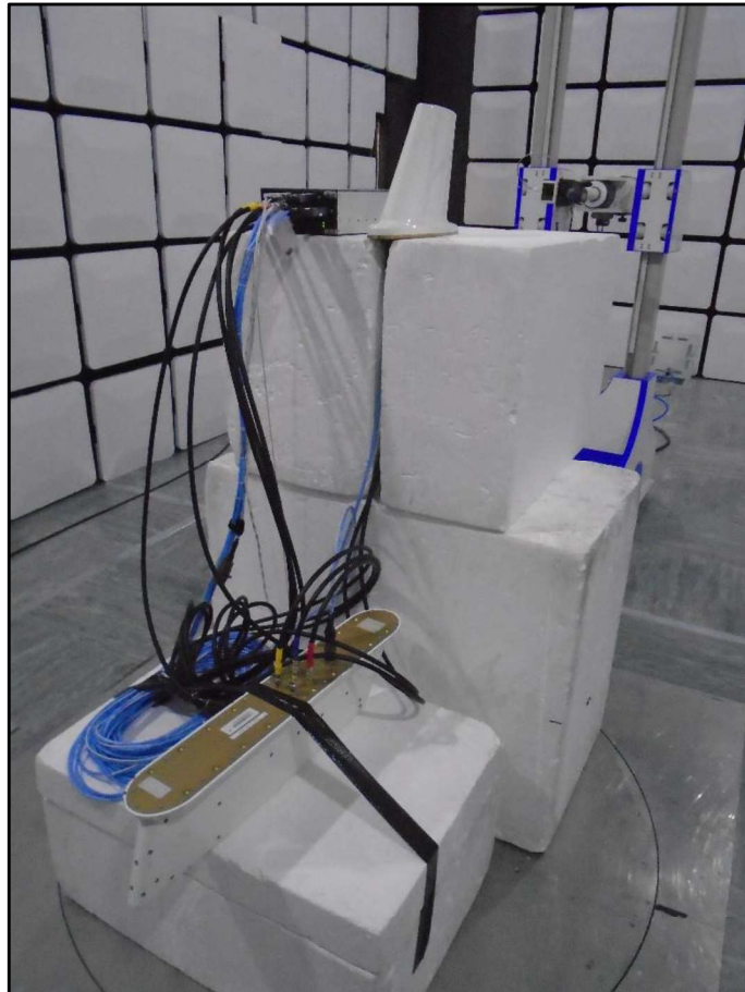
Figure 100 - Test Setup - 18 GHz to 25 GHz
