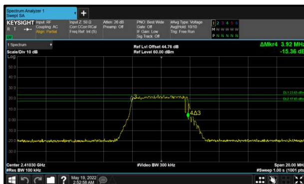
Figure 13 - LTE Full Resource Blocks 4.5 MHz BW Minimum 6 dB EBW
