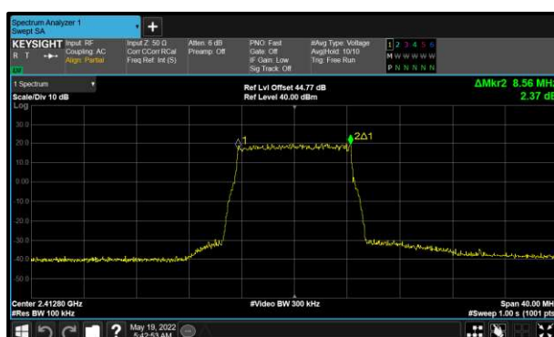
Figure 19 - LTE Full Resource Blocks 9 MHz BW Minimum 99% OBW
