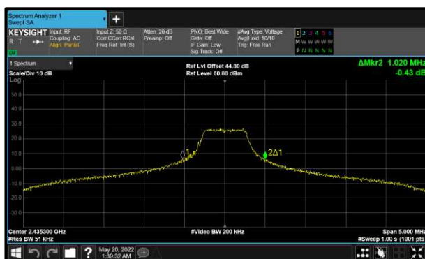
Figure 11 - LTE 3 Resource Blocks 4.50 MHz Minimum 99% OBW
