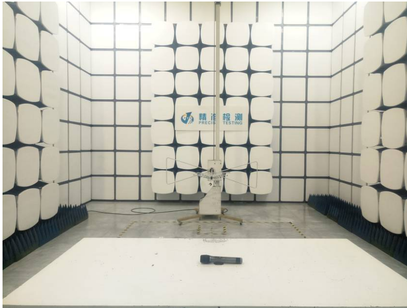
Radiated Spurious Emissions From 30MHz-1000MHz
