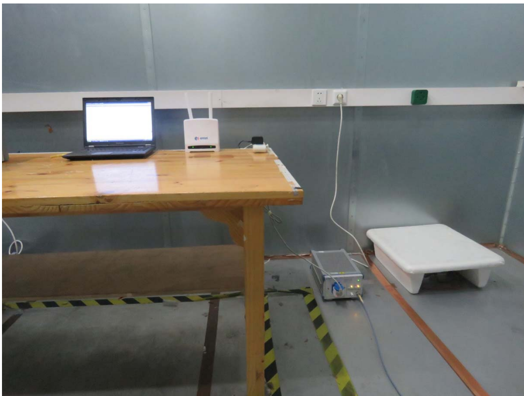
Picture 3 Conducted Emission Test Setup
