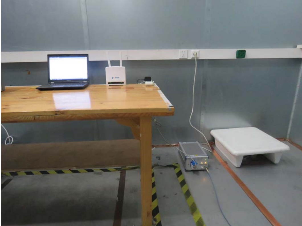
Conducted Emission Test Setup
