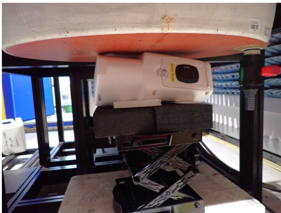
Figure D.4: EUT left face touching the body at 0mm gap configuration.
