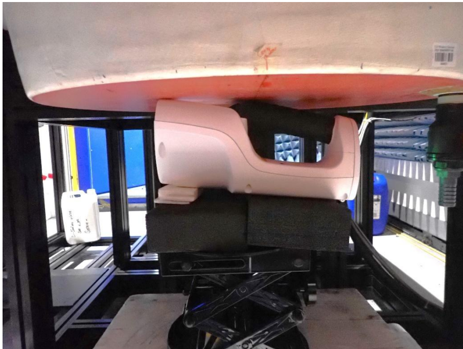
Figure D.7: EUT front face touching the body at 0mm gap configuration.
