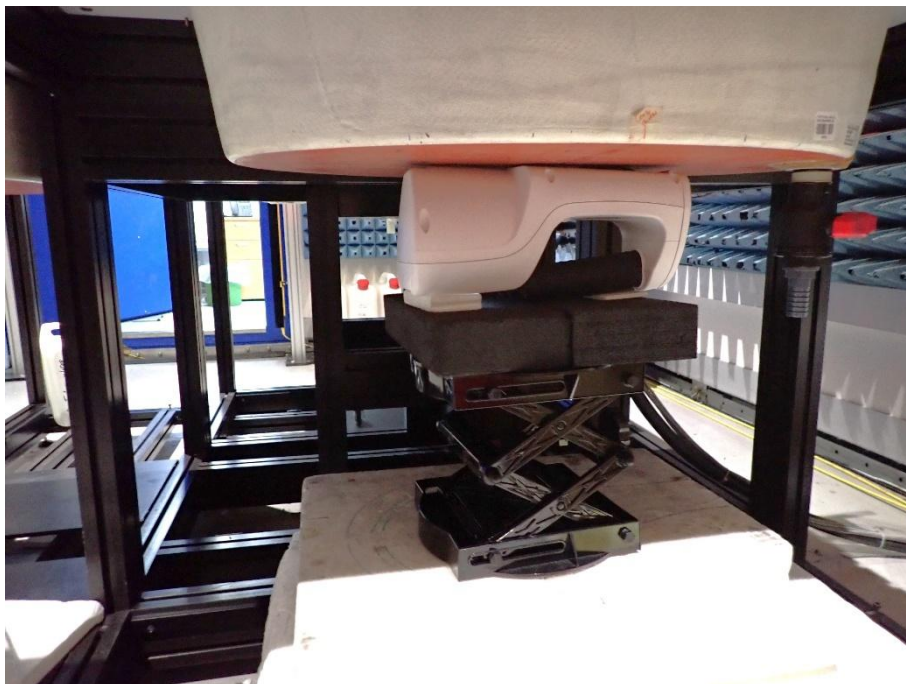
Figure D.8: EUT back face touching the body at 0mm gap configuration.
