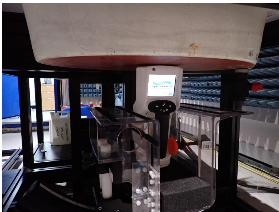
Figure D.6: EUT top face touching the body at 0mm gap configuration.
