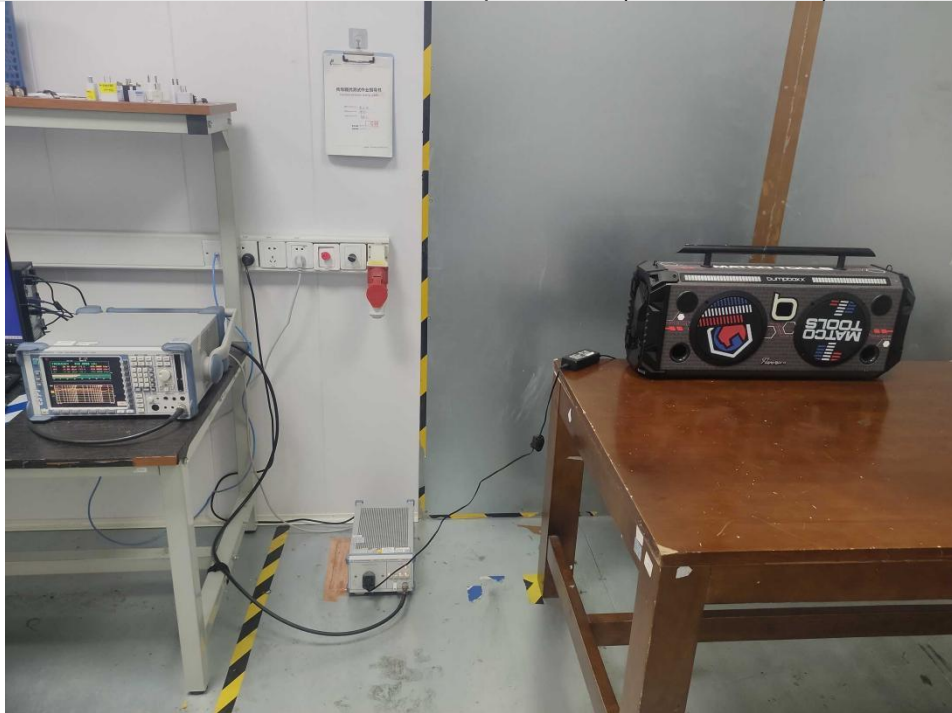
Conducted emissions at AC power line (150kHz-30MHz)
