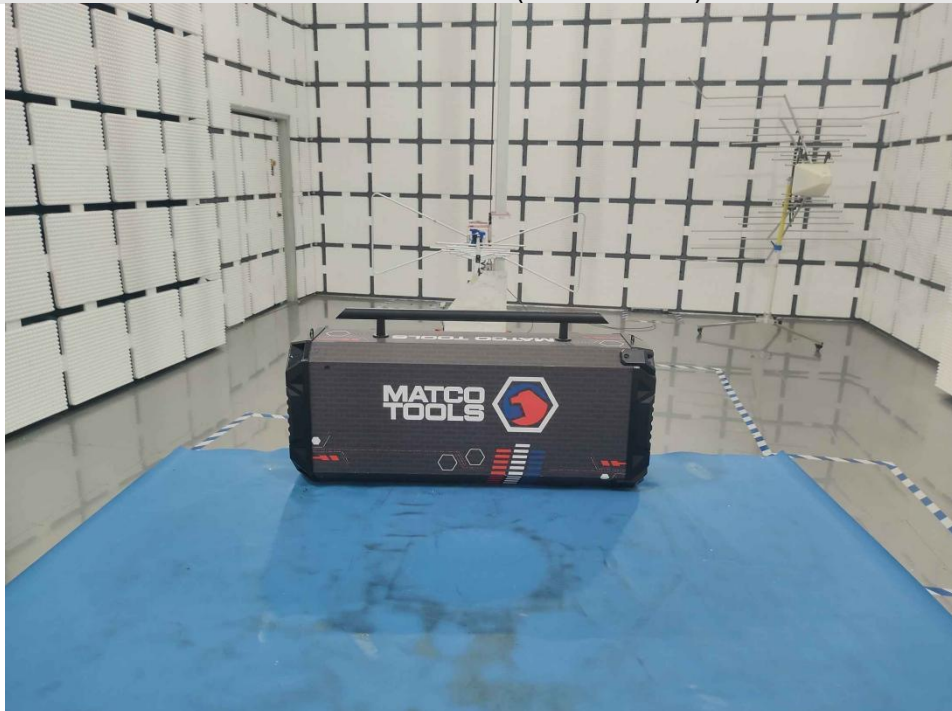
Radiated Emissions (30MHz-1GHz)
