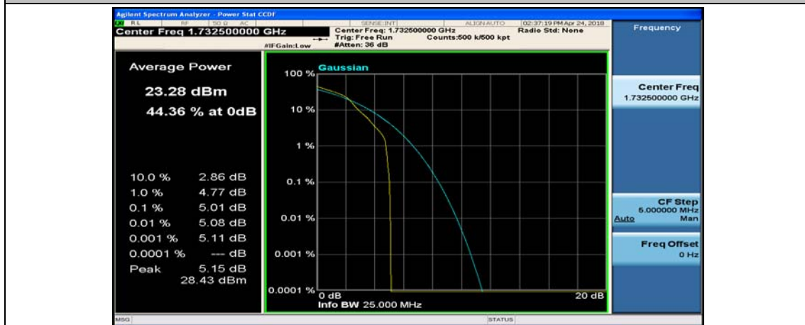
(Channel Bandwidth: 3 MHz)_MCH_16QAM_1RB#14
