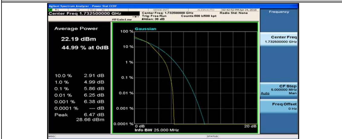
(Channel Bandwidth: 5 MHz)_MCH_16QAM_25RB#0
