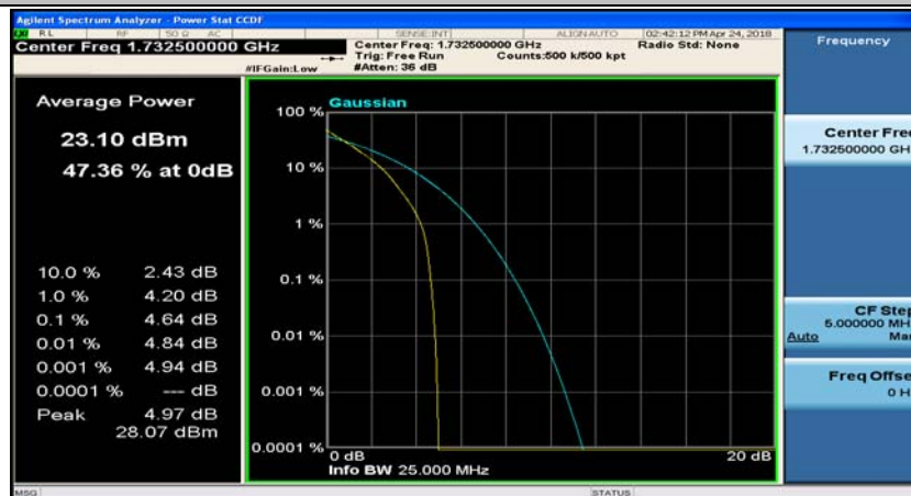
(Channel Bandwidth: 5 MHz)_MCH_QPSK_12RB#13
