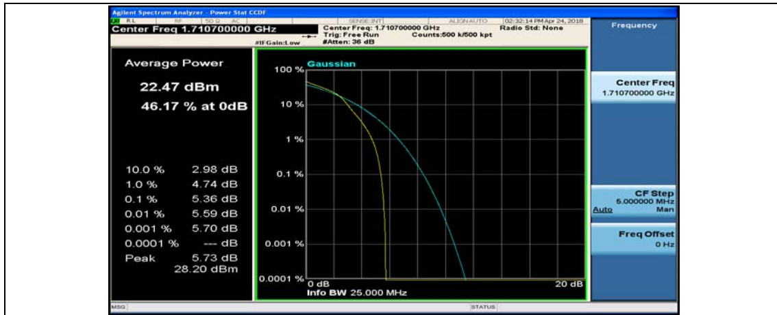
(Channel Bandwidth: 1.4 MHz)_MCH_16QAM_1RB#0
