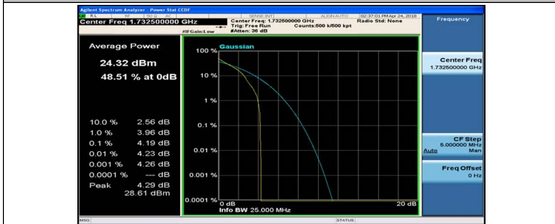
(Channel Bandwidth: 3 MHz)_MCH_QPSK_1RB#14
