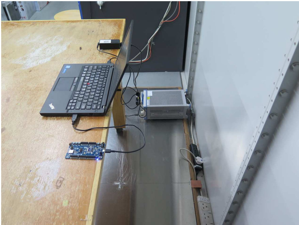
Line conducted emission (side view) (Data transfer)
