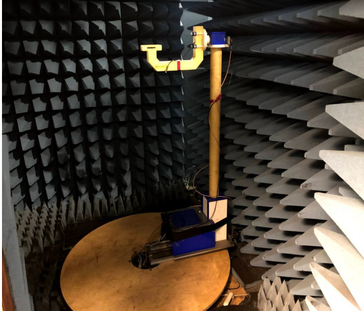
Figure 4. Receiving antenna in the anechoic chamber.
