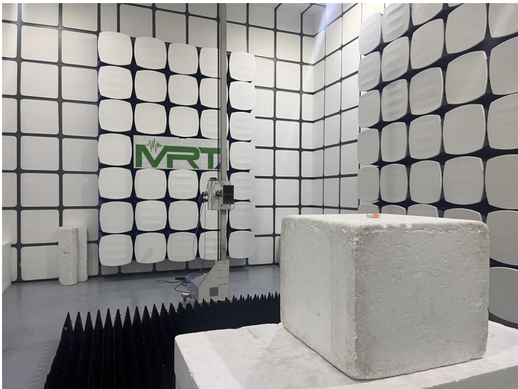
Description: Radiated Spurious Emission Test Setup for Above 1GHz(BLE)
