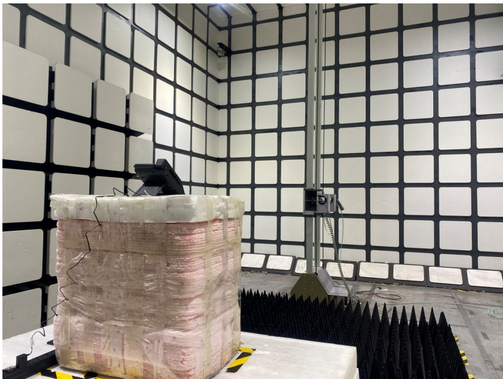
Radiated Emissions View (1-18 GHz)
