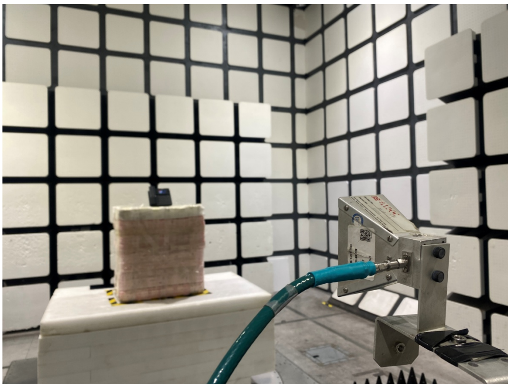
Radiated Emissions View (18-25 GHz)
