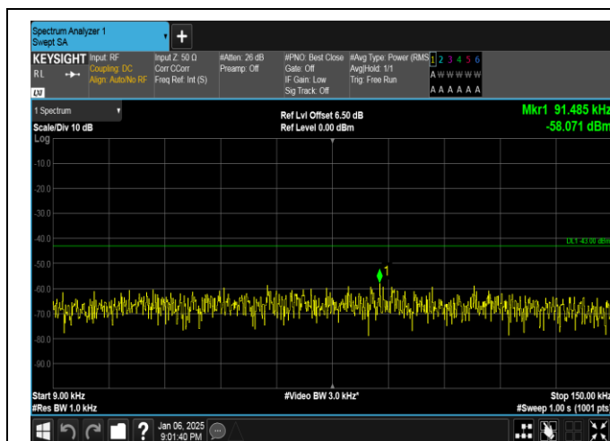
The screenshot displays the Keysight Spectrum Analyzer interface. The top panel shows various settings: Input RF, Coupling DC, Align Auto, Input Z 50 Ω, Corr CCoat, Freq Ref Int (S), Attain 30 dB, Preamp Off, PNO Fast Gate Off, IF Gate Low, Sg Track Off, Avg Type Power (RMS), Avg Hold 1/1, Trg Free Run, and a table of 23 data points (1 to 6 are visible, all showing 'A'). The main display area shows a spectrum plot with a green horizontal line at -30.00 dBm and a yellow trace at -63.054 dBm. The plot is labeled 'Mkr1 850.6 MHz' and '-63.054 dBm'. The bottom panel shows the start frequency at 0.0300 GHz, resolution bandwidth at 100 kHz, video bandwidth at 300 kHz, and sweep parameters: Stop 1.0000 GHz, #Sweep -1.00 s, and (2001 pts).
