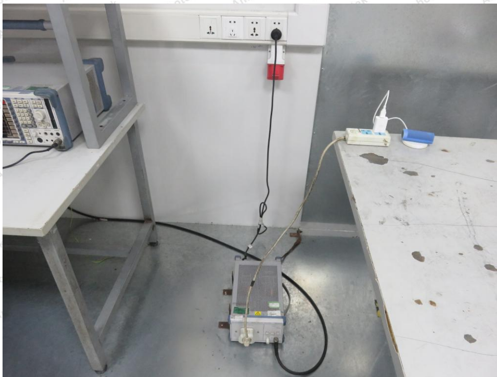
Photo of Power Line Conducted Emission Test
